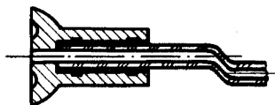
Fig. 18. Teflon O-ring joint with a cross-section of the joint with an inserted quartz tube.
