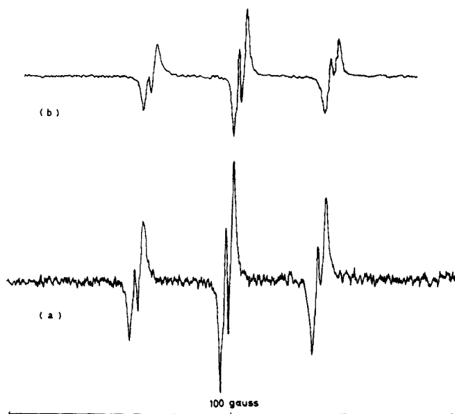
Fig. 2. E.s.r. spectra of bianthranyl + \text{NO}_3^- (a) and anthrone + \text{NO}_3^- (b) in 96 % \text{H}_2\text{SO}_4 (room temp.).
