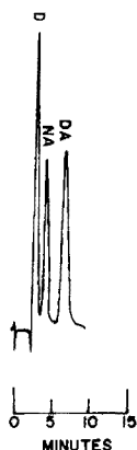
Fig. 2. Separation of biogenic amines with fluorescence detection of their o -phthalaldehyde derivatives. D = L-dopa, NA = noradrenalin, DA = dopamine.
