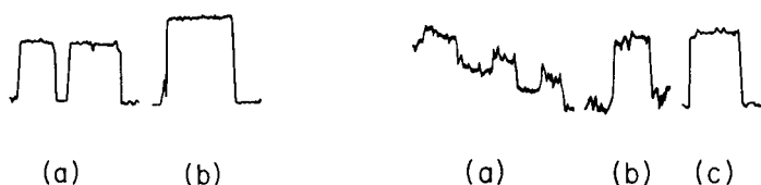
Fig. 5. (left). Non-dispersive atomic fluorescence signals from cadmium ( 2 \text{ ng ml}^{-1} ). (a) EDL, 7.5 W (repeated measurements); (b) boosted-output lamp, 10 mA/500 mA, electronically modulated.
