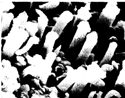
Fig. 4. Scanning electron micrographs of whiskers grown on the wall of a 2-mm i.d. Pyrex glass tube. Magnification: 2500 \times .
