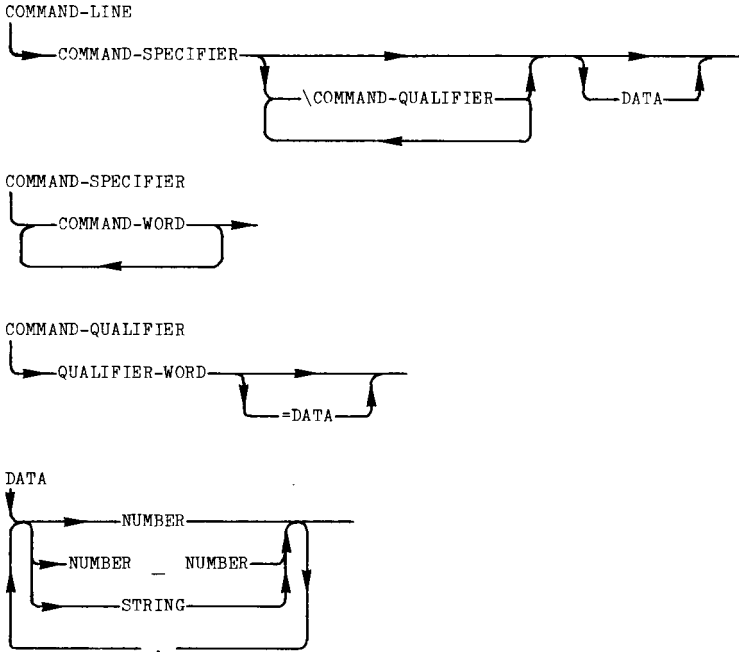
Fig. 1. Syntax diagram of the input command language implemented in DPP. This command language is used to control the operation of the program.
