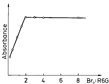
Fig. 3. Effect of the rhodamine 6G concentration on the formation and flotation of the gold compound (1 M \text{H}_2\text{SO}_4 during flotation): (1) absorbance of the gold compound solution against the blank; (2) blank against methanol.
