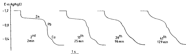
Fig. 4. Quasi-continuous monitoring of zinc, lead, and copper in tap water. Four characteristic potential/time curves taken during an uninterrupted 3-h period of analysis.
