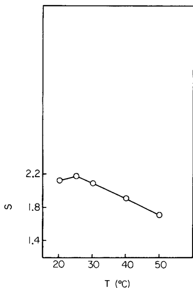
Fig. 2. Influence of the temperature on the fluorescence intensity of the aluminium/lumogallion complex in presence of Triton X-100. S, slope of calibration graph.
