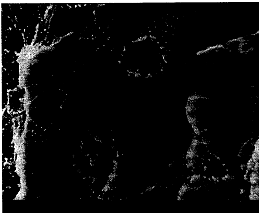
Fig. 7. SEM image of palladium domains on a L'vov platform using 20 \mu\text{l} of 0.1% tetraaminepalladium(II) chloride solution (modifier M-1). Dried and ashed until atomization step (Table 1). Area ca. 35 \times 25 \mu\text{m} .
