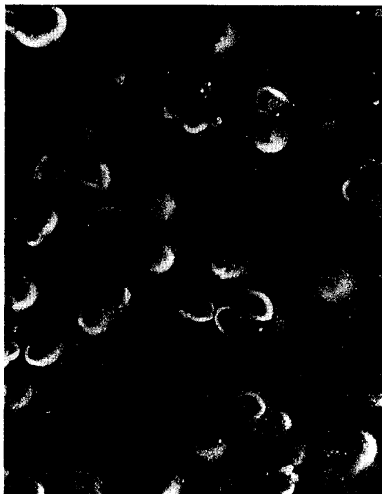
Fig. 2. (a) A scanning electron micrograph of a polypyrrole–nitrate film, prepared with 0.1 M \text{NaNO}_3 and 0.49 M pyrrole for 20 min with a 0.25 \text{ mA cm}^{-2} current density on gold coated plastic. Magnification 400\times . (b) Scanning electron micrograph of a polypyrrole–urease film, prepared from a 2000 \mu\text{g ml}^{-1} urease solution and 0.49 M pyrrole for 20 min with a 0.25 \text{ mA cm}^{-2} current density on a gold coated plastic. Magnification 400\times .
