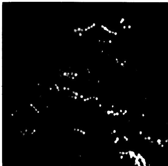
Fig. 2. An example of a measured image and its data processing for area distribution. Fluorescent latices were agglutinated with ac field. The area for each latex cluster was measured and the frequency distribution of each bead cluster was used to determine AR.
