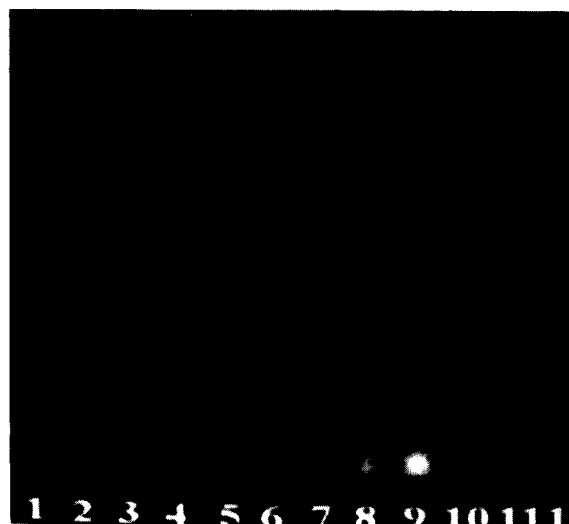
Fig. 7. A view reproduced from CCD of the TLC plate eluted in hexane–ether–ethanol solvent refilled five days after first exposure to excitation at 360 nm light and air. The spots at the start from left to right are (1) BCD in acetonitrile–water (25:75, w/w); (2) BCD in acetonitrile–water (38:62, w/w); (3) DPH in acetonitrile–water (25:75, w/w); (4) DPH + 4 \times 10 3 pmol BCD in acetonitrile–water (25:75, w/w); (5) DPH + 12 \times 10 3 pmol BCD in acetonitrile–water (25:75, w/w); (6) DPH + 20 \times 10 3 pmol BCD in acetonitrile–water (25:75, w/w); (7) DPH + 4 \times 10 3 pmol BCD in acetonitrile–water (38:62, w/w); (8) DPH + 12 \times 10 3 pmol BCD in acetonitrile–water (38:62, w/w); (9) DPH + 20 \times 10 3 pmol BCD in acetonitrile–water (38:62, w/w); (10) 50 pmol DPH standard. (11) 80 pmol standard. (12) 100 pmol standard. All DPH standards are in pure acetonitrile.
