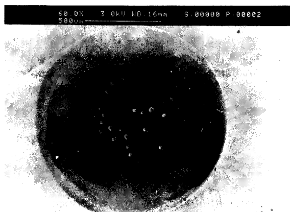
Fig. 2. Photograph of a Sephadex modified carbon paste electrode. The small round particles are the AH Sephadex grains.
