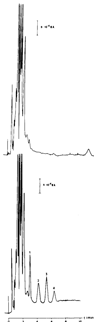
Fig. 4. Chromatogram of a processed meat sample and a spiked sample at ppb levels (5–7 ng g -1 ). (1) B(c)Ac; (2) DB(aj)Ac; (3) DB(ac)Ac; (4) DB(ch)Ac.
