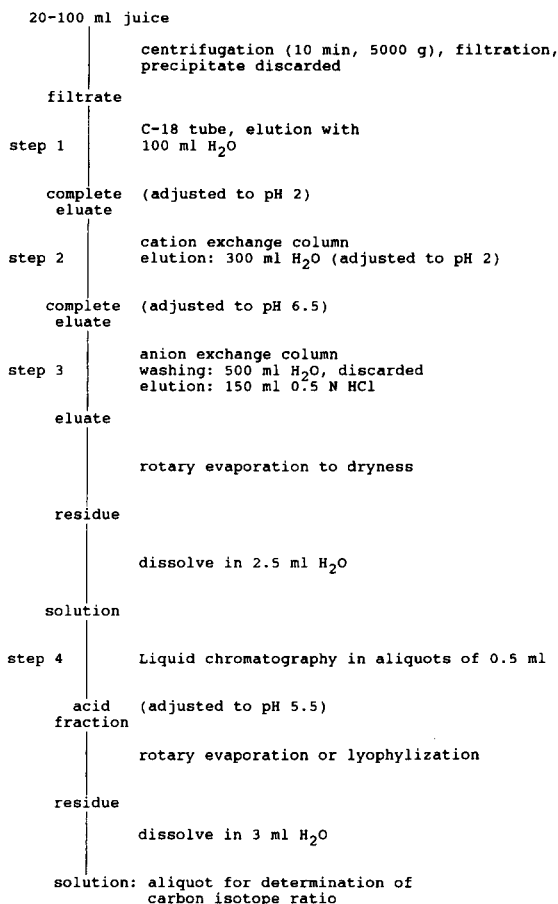
Fig. 1. Diagram for the isolation of the main organic acids (CA, L-MA, L-TA) from juices for carbon isotope ratio measurements. Step means chromatographic procedure.
