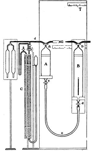
B, and displaces an equal volume of water through the upper three-way tap b. This tap is then closed, and the bulb B is raised to the position indicated at T;
