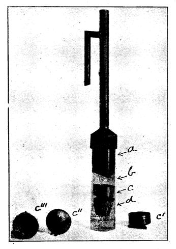
twenty analyses may be conducted simultaneously on an electric hot plate,  $4\frac{1}{2}$  ins.  $\times 24$  ins. About 15 c.c. of ether are used, of which one-third to one-half is
