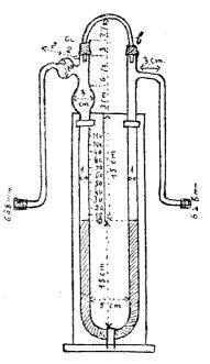
sponding with the deviations in level h. It is essential that the gas should be dry. Changes of temperature are corrected by means of the formula—
