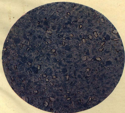
Fig. 5. Ultramarine from Lapis Lazuli, \times 200 .
