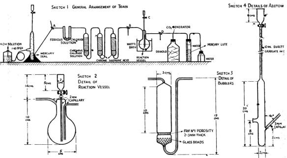
APPARATUS—The azotometer has a capacity of 10 ml. The three gas-washing tubes should have sintered glass discs of No. 1 porosity. Sintered discs are essential to ensure complete removal of oxides of nitrogen. The U-tube should be packed with broken glass rod or beads. Some form of carbon dioxide generator is required. That illustrated is for use with Drikold; any form of generator suitable for the micro-Dumas procedure could be used, but it must give a pressure equiv. to ca. 5 cm of mercury.
