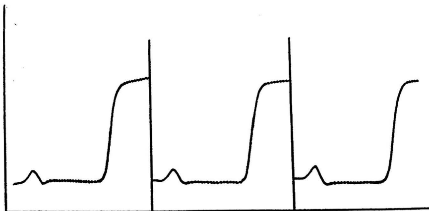
Fig. 14 (c). Differential polarograms of zinc + cadmium in 0.5 M ammonium chloride + 0.5 M ammonium hydroxide + 0.01 per cent. gelatin solution. S = \frac{2}{3} . 8 \times 10^{-5} M zinc + 2 \times 10^{-3} M cadmium
