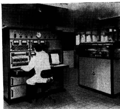
MASS SPECTROMETER TYPE MS5 An instrument specially designed for the measurement of isotope ratios of inorganic solids by the surface ionisation technique.
