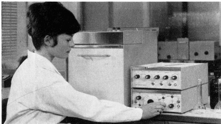
Oven accommodates interchangeable head units incorporating different detector and column configurations and is designed for isothermal or programmed temperature control.
