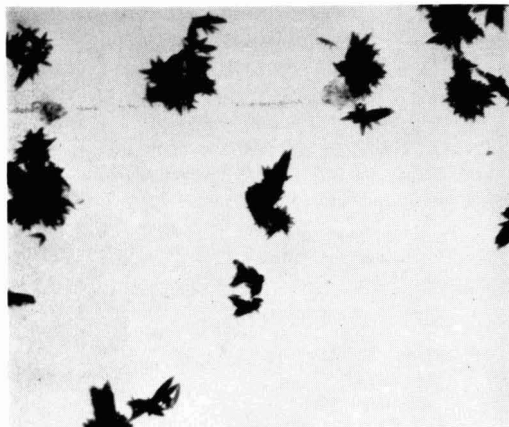
Fig. 1. Electron photomicrograph of aragonite crystals precipitated at 35° C in Run 15, indicating small unclustered particles. Magnification, \times 5000
