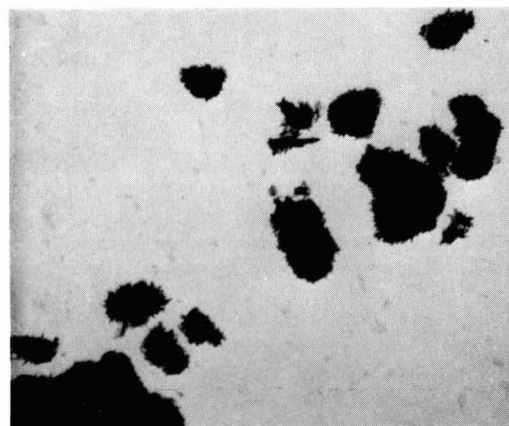
Fig. 3. Electron photomicrograph of calcite crystals from Run 7. Magnification, \times 5000
