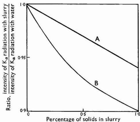
Fig. 1. Effect of change in particle size on back-scattered cadmium  $K_{\alpha}$  intensity: curve A, particles from 100 to 150 mesh; curve B, particles less than 300 mesh
