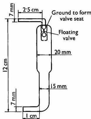
Fig. 6. Potassium thiocyanate vessel
