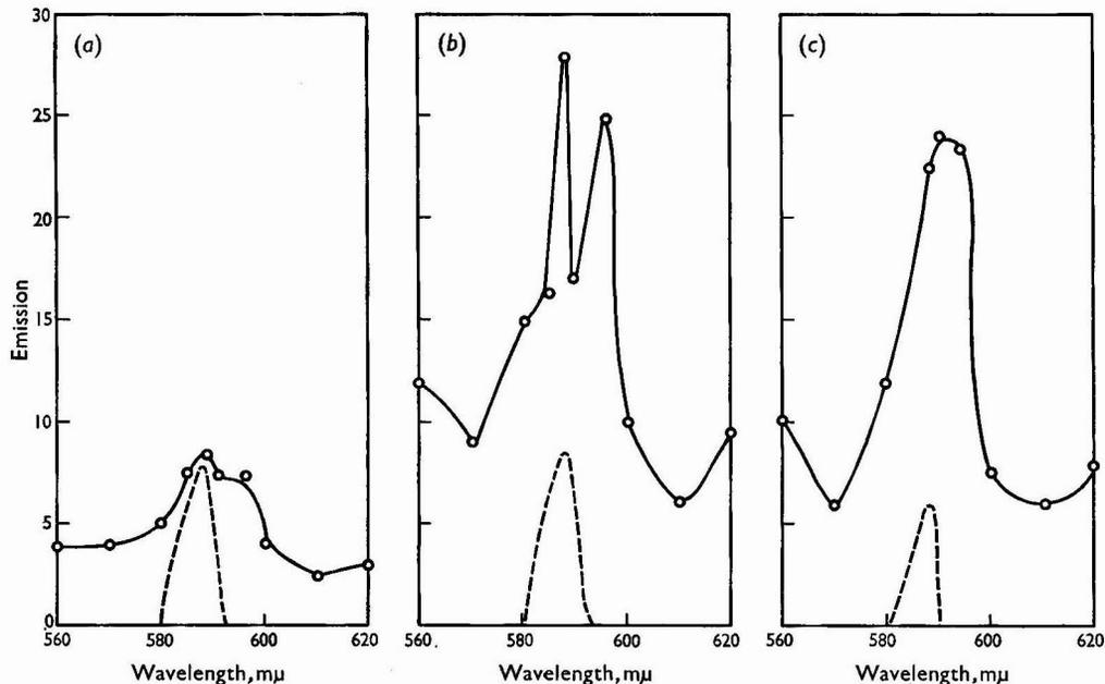
Fig. 3. Spectra of solutions before and after extraction of iron (10 mg per 100 ml). Broken lines, iron-free spectrum; continuous line, iron with sodium impurity. (a) air pressure, 23 p.s.i.; acetylene pressure, 14 cm; (b) air pressure, 23 p.s.i., acetylene pressure, 8 cm; (c) air pressure, 23 p.s.i., acetylene pressure, 4 cm
