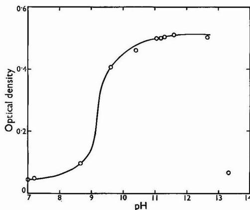
Fig. 2. Effect of pH on the determination of 4.74 p.p.m. of oleic acid
