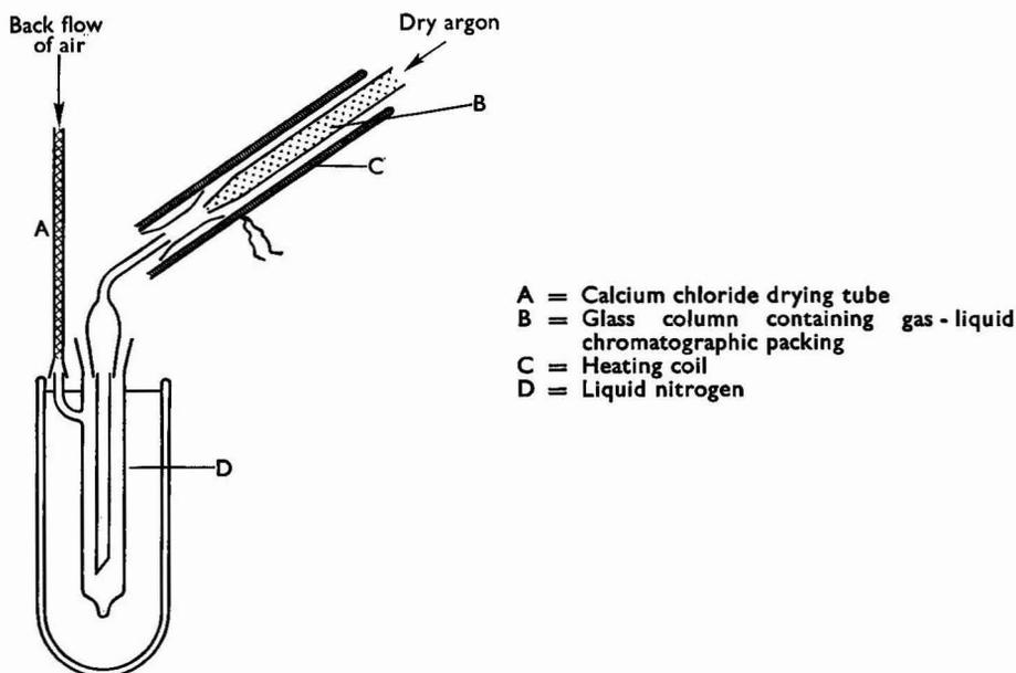
Fig. 1. Apparatus for the column packing, total-trapping technique
