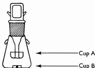
Fig. 1. Modification of the Cavett flask used for micro diffusion work (quarter scale)
