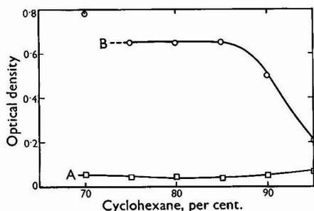
Fig. 1. Effect of addition of cyclohexane to the isobutanol extractant: curve A, blank; curve B, sample corrected for blank
