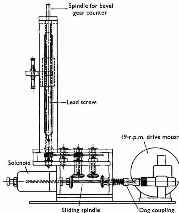
Fig. 7. Two-speed gearbox
