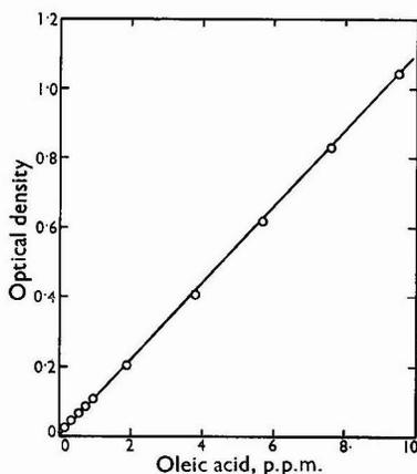
Fig. 5. Calibration for oleic acid
