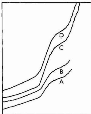
Fig. 1. Polarographic determination of arsenic in 0.4000 g of NBS steel, No. 464-D. Curves A and B, arsenic content of sample; curves C and D, arsenic found after addition of standard. Polarographic conditions: Radiometer PO 3h polarograph,  $V = 2$  ml (from 25 ml),  $V_s = 0.05$  ml,  $C_s = 1.5 \times 10^{-4}$  g per ml, sensitivity =  $1 \times 100$
