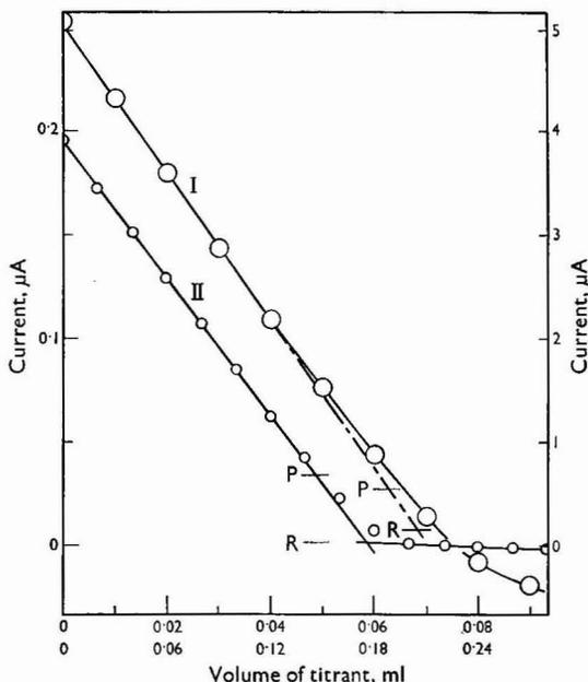
Fig. 1. Pre-addition titration of iodine in sulphuric acid and 0.02N potassium iodide. P and R are the pre-addition and residual current lines, respectively. Iodine, sulphuric acid and approximate titrant normalities are, respectively: curve I,  $2.6 \times 10^{-6}$ , 0.1, and 0.002 (left ordinate and upper abscissa); curve II,  $5 \times 10^{-5}$ , 5.0, and 0.02 (right ordinate and lower abscissa)
