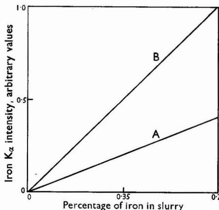
Fig. 2. Effect of change in particle size on iron  $K_{\alpha}$  intensity from the slurry: curve A, particles from 100 to 150 mesh; curve B, particles less than 300 mesh
