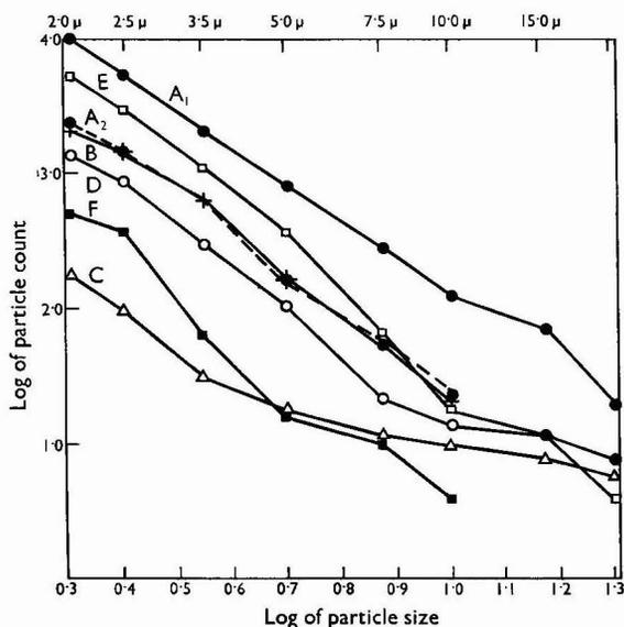
Fig. 3. Particle-size distribution for samples of: curve A<sub>1</sub>, 0.9 per cent. sodium chloride solution; curve A<sub>2</sub>, potassium-free maintenance fluid; curve B, 4.3 per cent. dextrose in 0.18 per cent. sodium chloride solution; curve C, Darrow's solution; curve D, tissue repair solution, No. 1; curve E, 5.0 per cent. dextrose in 0.9 per cent. sodium chloride solution; curve F, 0.9 per cent. sodium chloride solution
