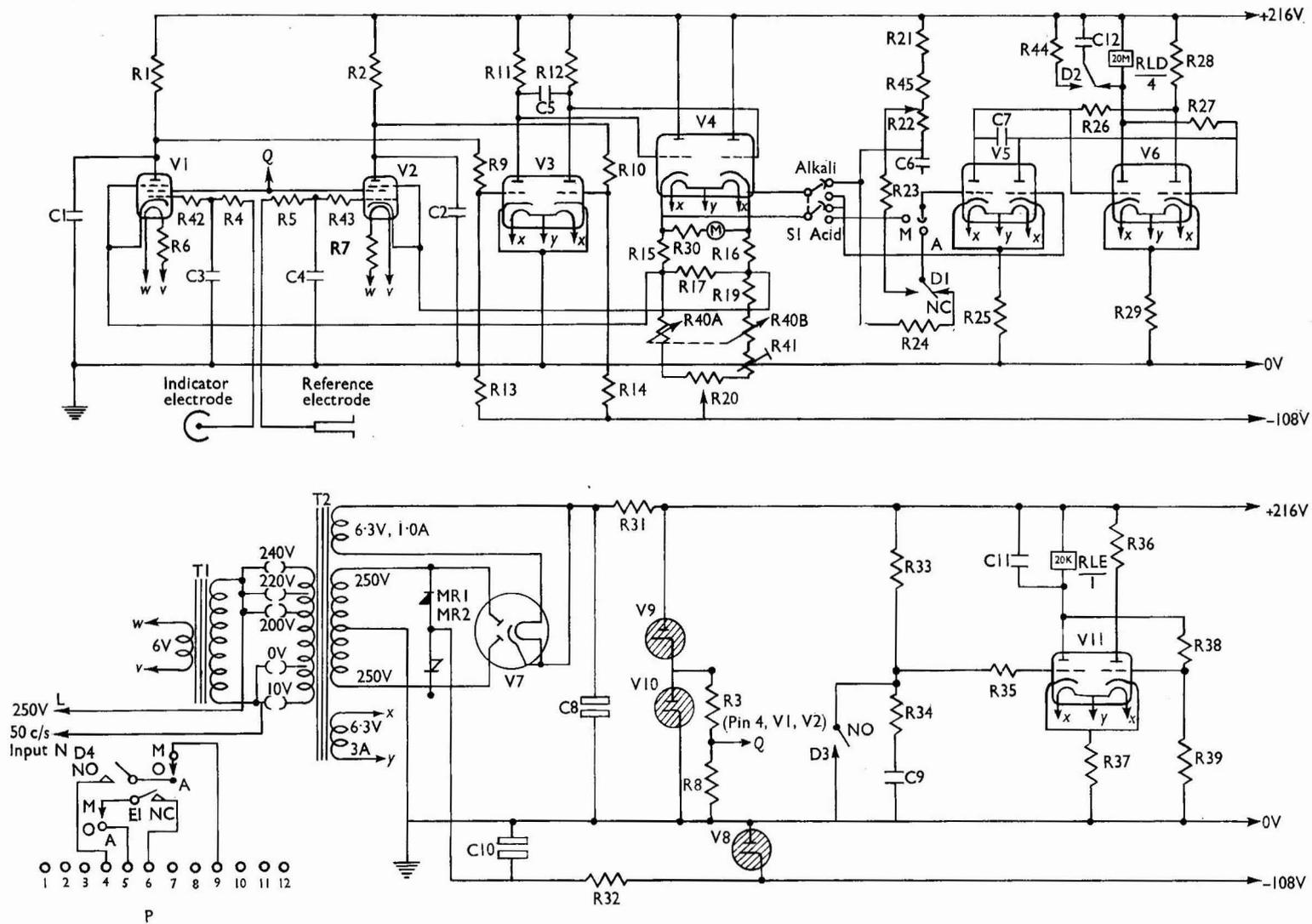
Fig. 1. End-point detector circuit diagram
