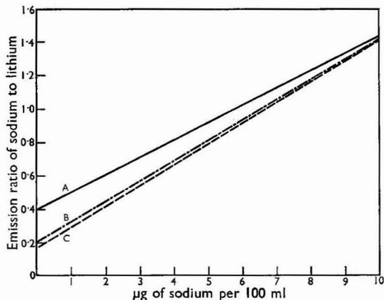
Fig. 2. Calibration graphs for different flame conditions. Acetylene pressure: (A) 8 cm; (B) 14 cm; (C) 4 cm
