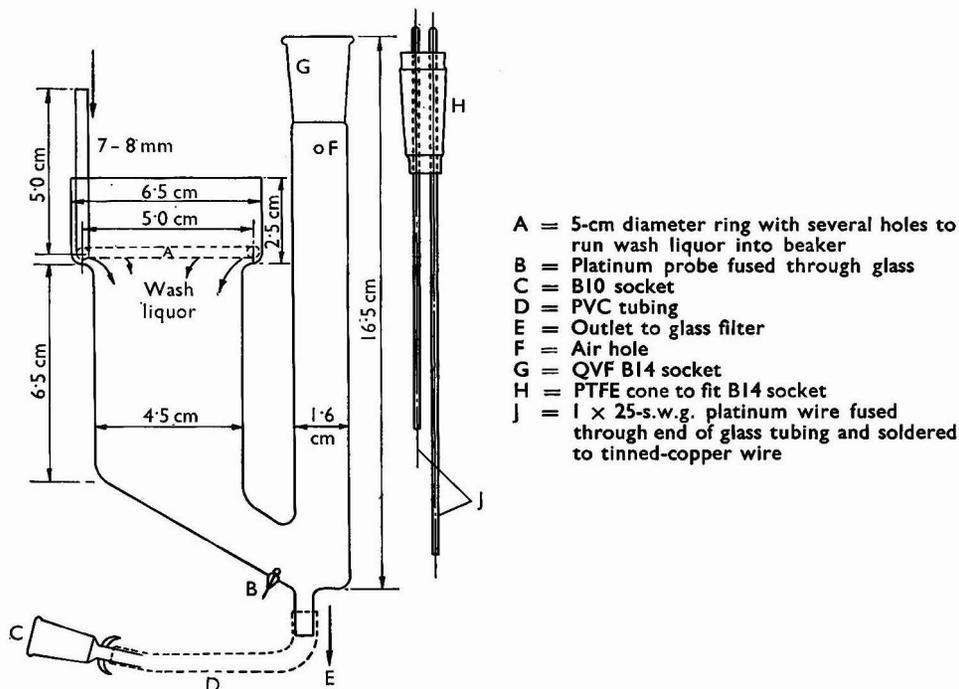
Fig. 2. Sample beaker and probes
