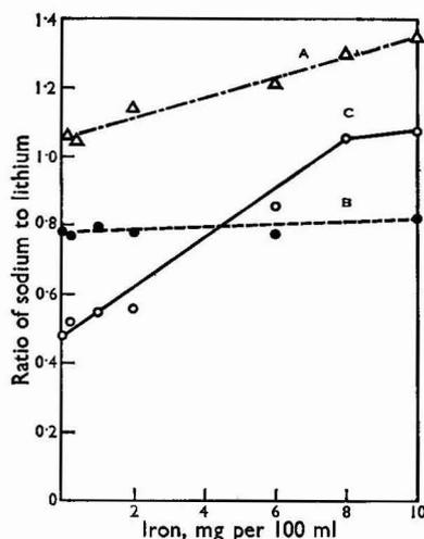
Fig. 4. Effect of increasing iron on emission of 5  $\mu$ g of sodium per 100 ml. Acetylene pressure: Graph A ( $\Delta$ ), 8 cm; graph B ( $\bullet$ ), 14 cm; graph C ( $\circ$ ), 4 cm
