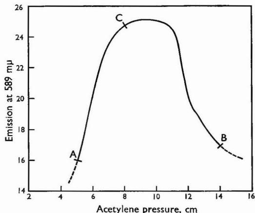
Fig. 1. Effect of flame condition on background emission at 589  $m\mu$ . A: Air-rich and unstable flame; B: Fuel-rich flame and C: Balanced flame
