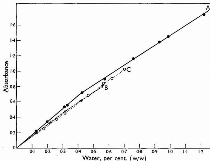
Fig. 1. Beer's Law relationships for water in lubricating oil samples. Graph A, in ethyl acetate; graph B, in ethyl acetate and straight oil, 2 to 1, v/v; graph C, in ethyl acetate and detergent oil, 2 to 1, v/v
