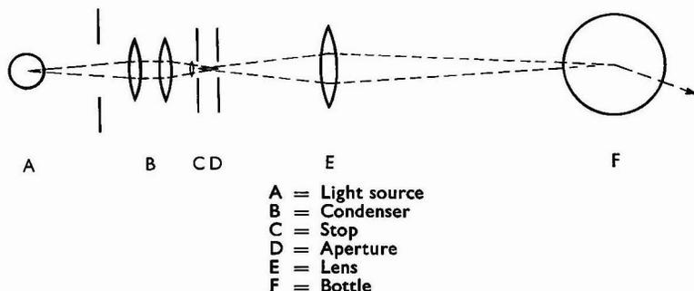
Fig. 1. Light-scattering apparatus for the visual detection of small particles
