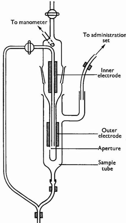
Fig. 2. Sample vessel for Coulter Counter
