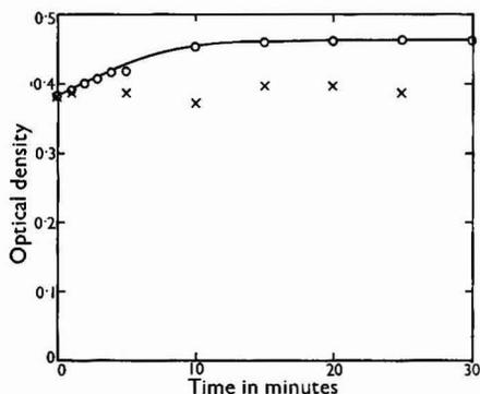
Fig. 3. Development of copper(II) dithiocarbamate colour: O, protected from light; X, exposed to light
