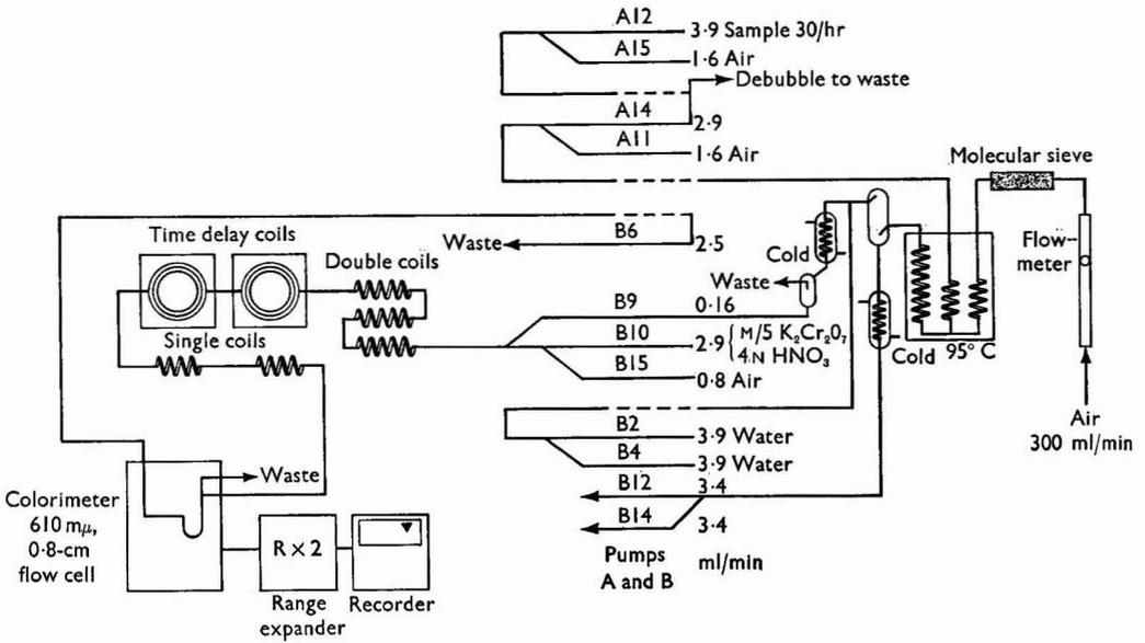
Fig. 2. Manifold for alcohol
