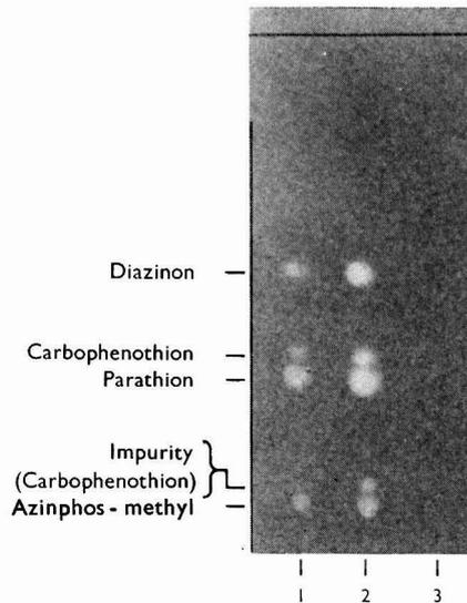
Fig. 4. Chromatogram of fortified and control eluate B of potato and corresponding standard. (Concentrations are given in Table II.) 1, 10  $\mu$ l of eluate B fortified with pesticide standard mixture at B<sub>2</sub> concentration (equivalent to 10 mg of sample); 2, 10  $\mu$ l of pesticide standard mixture at B<sub>2</sub> concentration; 3, 10  $\mu$ l of control eluate B (equivalent to 10 mg of sample)
