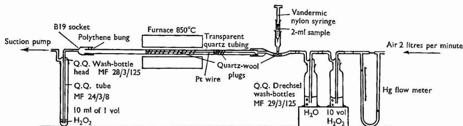
Fig. 1. Modified Schöberl surface combustion apparatus
