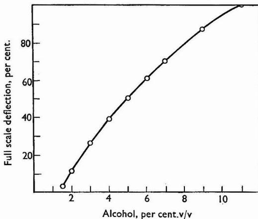
Fig. 6. Calibration curve of ethanol, per cent., against full scale deflection
