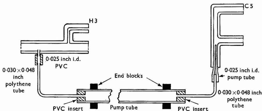
Fig. 1. Connection of debubbler to pump tube and return to manifold for dilution
