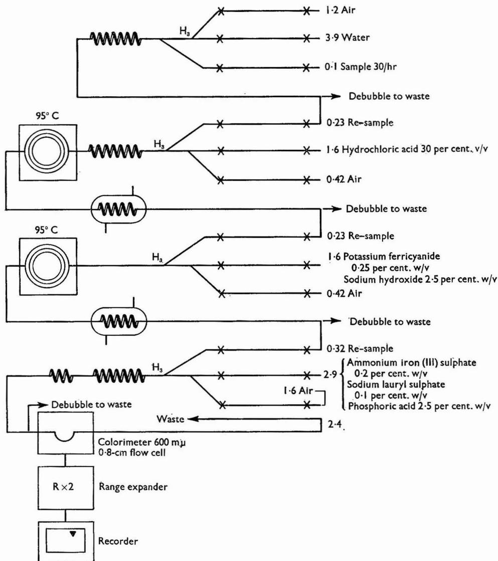
Fig. 2. Manifold for the total hydrolysable sugars in beer by the Prussian blue method
