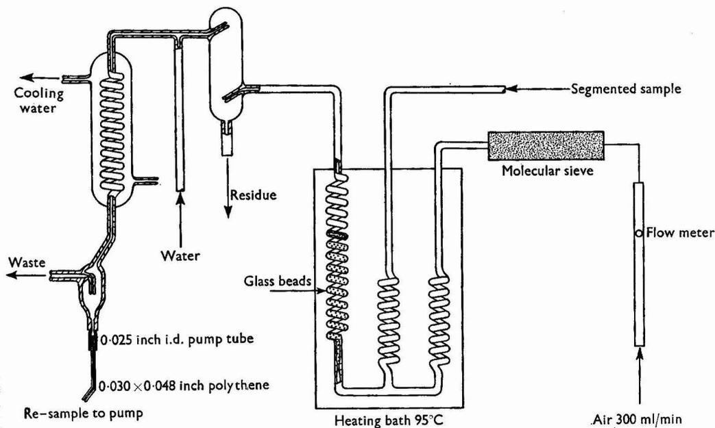
Fig. 1. Distillation flow path
