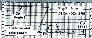
greatly increases the readability of a polarogram. **Below:** Normal DC-Polarogram of brass dissolved in  $\text{KNO}_3$ . The Pb-step is hardly discernible. **Above:** In tast polarography with controlled drop life, the step can be enlarged 50 times in a horizontal direction.
