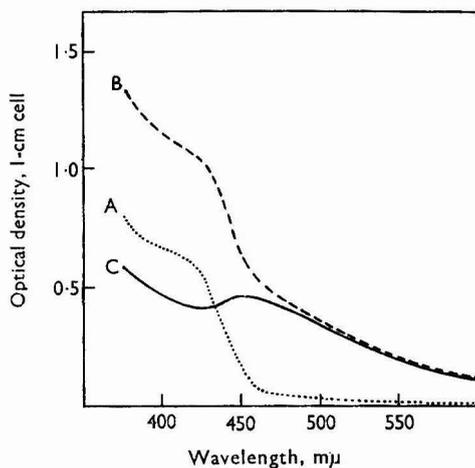
Fig. 6. Spectrum plots of molybdophosphoric acid-ferrocyanide system for: A, reagents against water; B, reaction mixture for 10 per cent. sugar against water; C, reaction mixture against reagents
