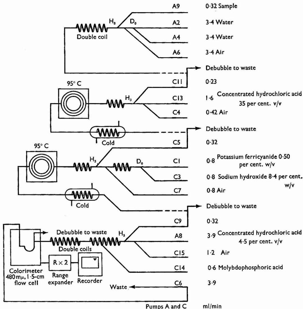
Fig. 7. Manifold for total hydrolysable sugars in beer
