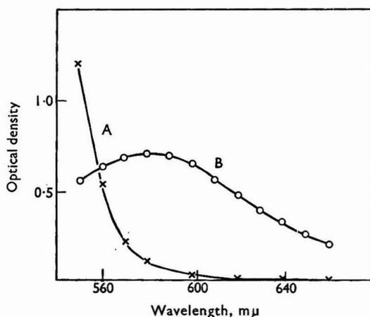
Fig. 4. Spectrum of alcohol reagent system for A, reagents against water; B, reagents plus 11 per cent. of ethanol against water in a 1-cm cell
