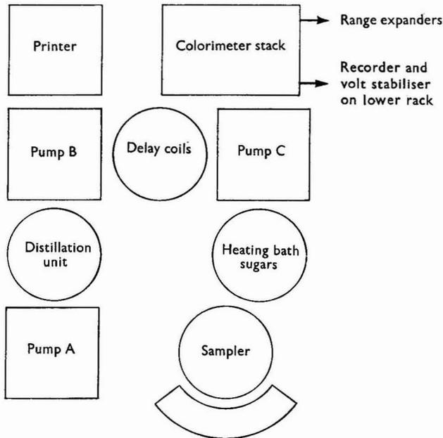
Fig. 3. Block schematic layout of operating units of AutoAnalyzer assembly for combined manifold
