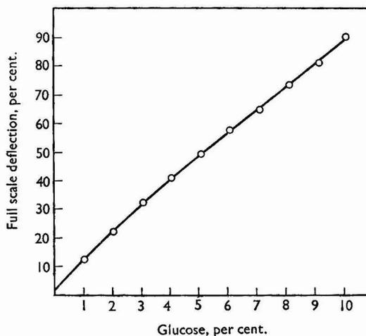
Fig. 4. Calibration curve, Prussian blue finish, of sugar as glucose, per cent. w/v, against full scale deflection, per cent.
