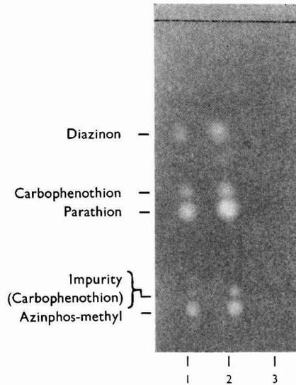
Fig. 3. Chromatogram of fortified and control extract B of potato and corresponding standard. (Concentrations are given in Table II.) 1, 10  $\mu$ l of extract B fortified with pesticide standard mixture at B<sub>2</sub> concentration (equivalent to 10 mg of sample); 2, 10  $\mu$ l of pesticide standard mixture at B<sub>2</sub> concentration; 3, 10  $\mu$ l of control extract B (equivalent to 10 mg of sample)
