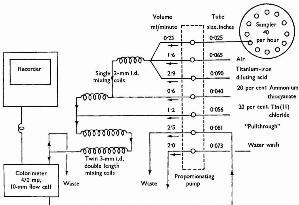
Fig. 1. AutoAnalyzer flow system for the determination of molybdenum in steel
