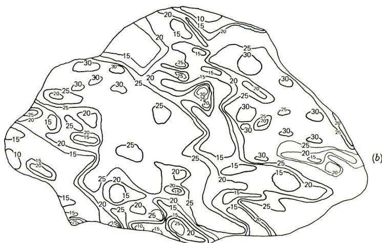
Fig. 3. (a), Section of copper pyrites sample; and (b), contour plan of intensity of \alpha -particles scattered from copper pyrites sample. Numbers given are thousands of counts recorded
