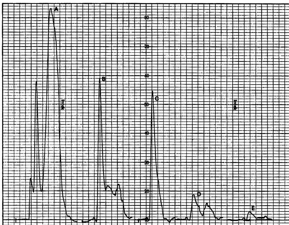
Fig. 2. Effect of iron and nitric acid background on the lead atomic-absorption signal: A, 0.1 p.p.m. of lead in 10 000 p.p.m. of iron and 8 per cent. nitric acid without background correction; B, as A but with background correction; C, as B but without iron; D, as B but without lead; and E, as B but without lead and iron.
