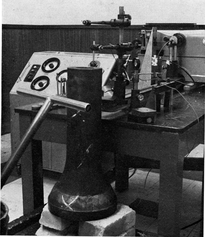
Fig. 5. Analysis of a large forging using a silica fibre-optic coupling between the excitation source and a photographic spectrograph.
