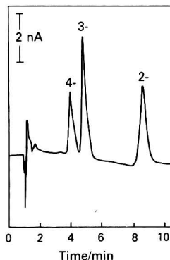
Fig. 5. Separation of a 10-ng mixture of 2-, 3- and 4-chloroaniline by HPLC with voltammetric detection. Flow-rate, 2 \text{ ml min}^{-1} ; applied potential, +1.2 V.
