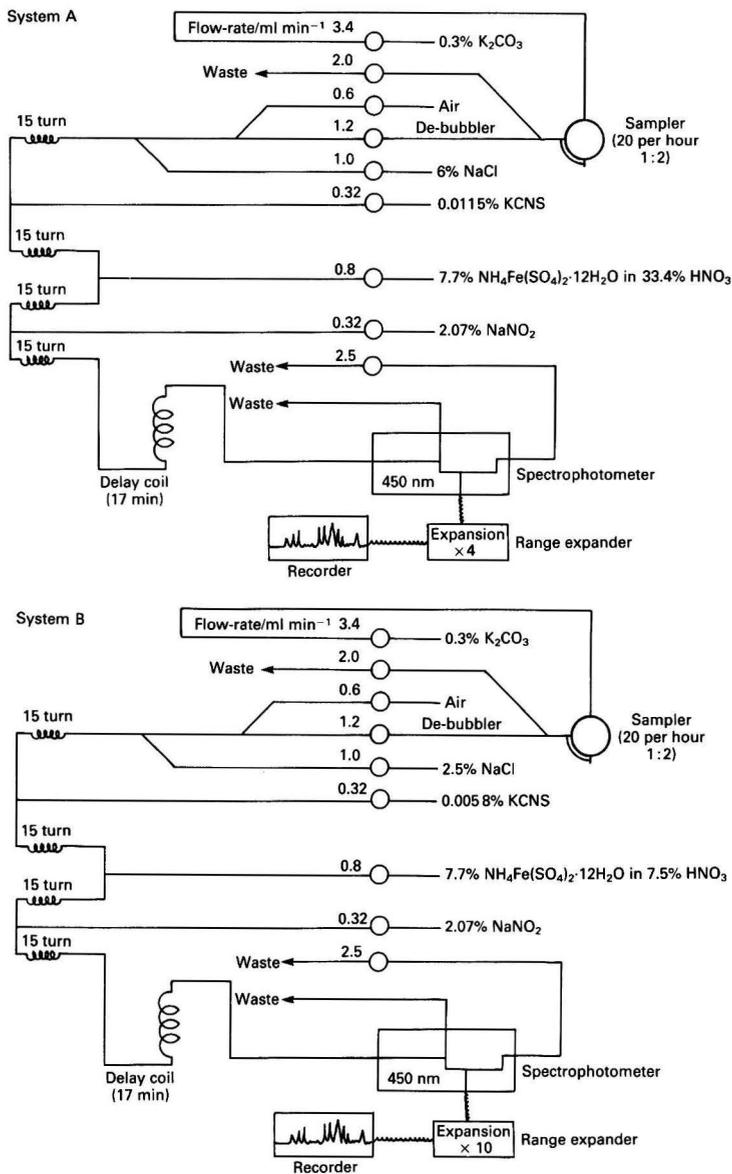
Fig. 1. Flow diagrams for the determination of total inorganic iodine in waters (system A) and free iodide in waters (system B)
