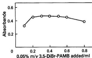
Fig. 3. Effect of reagent concentration on the formation of vanadium(V) complex; concentration of vanadium(V),  $0.4 \mu\text{g ml}^{-1}$
