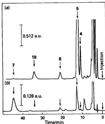
Fig. 3. HPLC of the mother liquor after crystallisation of hexachlorobenzene. Column: S5 ODS, 150 × 4.6 mm i.d. with a 50 × 4.6 mm i.d. pre-column. Injection: 20  $\mu$ l as a 1% solution in dichloromethane. Solvent: 85% aqueous methanol, 1 ml min<sup>-1</sup>, room temperature. Detectors: (a) 220 nm; (b) 270 nm. Numbering of compounds as in Table 1
