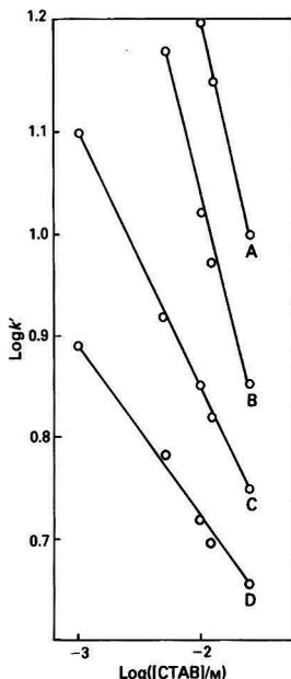
Fig. 2. Variation of log capacity factor ( $k'$ ) with log concentration of hexadecyltrimethylammonium bromide. (A) Sodium *N,N*-diethyldithiocarbamate; (B) ammonium tetramethylenedithiocarbamate; (C) sodium *N,N*-dimethyldithiocarbamate; and (D) sodium *N*-methyldithiocarbamate
