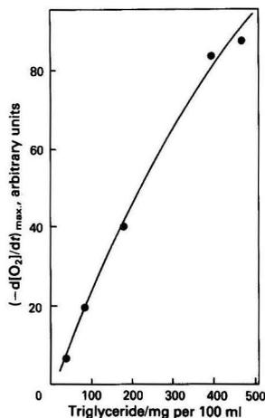
Fig. 7. Calibration graph for the determination of triglycerides in standard aqueous samples (by the external hydrolysis procedure)
