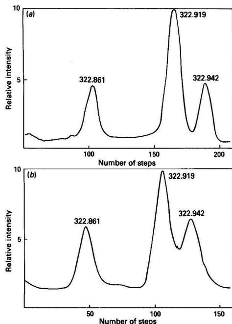
**Fig. 1.** Spectral scans of a  $10 \mu\text{g ml}^{-1}$  titanium solution. (a) Recorded with the scanning monochromator: dispersion  $0.42 \text{ nm mm}^{-1}$ ; theoretical resolution  $82\,500$ ; and observed spectral band pass  $0.022 \text{ nm}$ . (b) Recorded with the spectrograph and microdensitometer: dispersion  $0.50 \text{ nm mm}^{-1}$ ; theoretical resolution  $228\,000$ ; and observed spectral band pass  $0.031 \text{ nm}$ . Wavelengths, in nanometres, are indicated on the peaks
