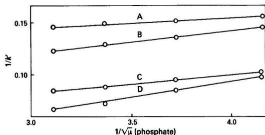
Fig. 5. Variation of capacity ratio with ionic strength. Mobile phase conditions: 70 + 30 V/V methanol - water;  $1.25 \times 10^{-2}$  M CTAB; flow-rate, 2 ml min<sup>-1</sup>, pH, 6.8 (phosphate buffer 0.018 M); and ionic strength control with phosphate. A-D as in Figs. 2 and 4
