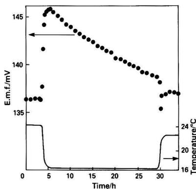
Fig. 4. Anomalous temperature response of aged electrode (D) in acetate buffer
