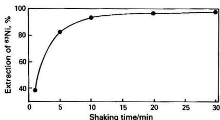
Fig. 1. Effect of shaking time with a wrist-action shaker at ca. 10 Hz on the extraction into the organic phase of <sup>63</sup>Ni added to plant digests. <sup>63</sup>Ni added at 7.6 kBq per sample; extraction pH, 4.0; and APDC-IBMK extracts counted in a 1 + 1 Triton-toluene mixture containing 0.5% m/V of 2,5-diphenyloxazole (PPO) on a Beckman LS100 liquid scintillation counter
