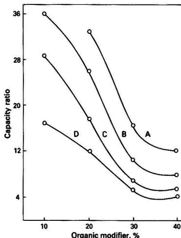
Fig. 4. Variation of capacity ratio ( $k'$ ) with concentration of organic modifier (methanol). (A) Sodium *N,N*-diethyl-dithiocarbamate; (B) ammonium tetramethylenedithiocarbamate; (C) sodium *N,N*-dimethyldithiocarbamate; and (D) sodium *N*-methyldithiocarbamate
