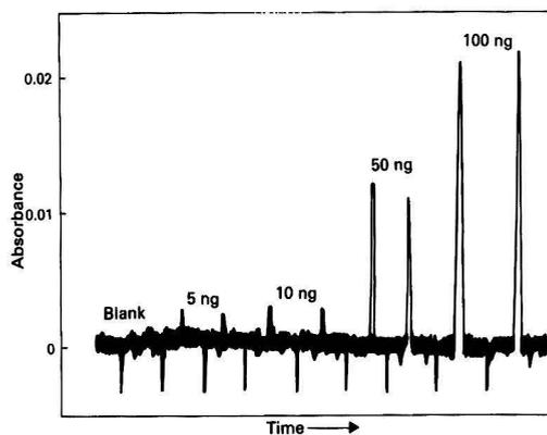
**Fig. 2.** Recorder tracings obtained from chloroform extracts with various mercury concentrations (20-µl aliquot in the furnace)
