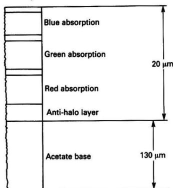
Fig. 3. Cross-section of a typical colour reversal film
