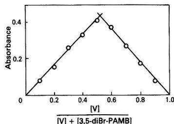
Fig. 4. Composition of vanadium(V) complex by the continuous variations method. Vanadium(V) complex in aqueous acetone solution: pH, 2.8; wavelength, 640 nm; and concentration,  $8 \times 10^{-5} \text{ M}$
