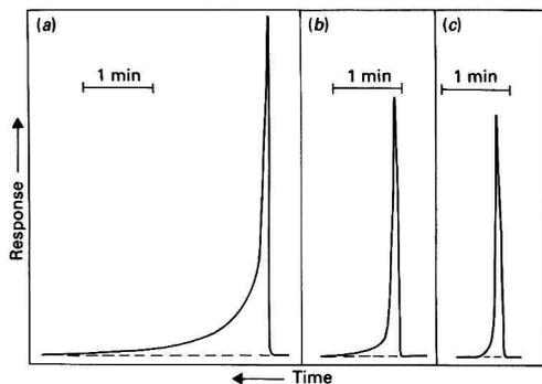
**Fig. 4.** Effect on sample rate of the addition of trace amounts of cyanide to the reagent stream. (a) No cyanide; (b) 0.2 p.p.m.; and (c) 0.4 p.p.m.
