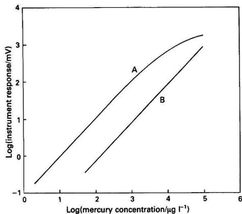
Fig. 1. ICP-AES calibrations for mercury, showing the enhancement in sensitivity produced by the addition to the test solution of tin(II) chloride. A, With 0.5% tin(II) chloride added; and B, normal nebulisation
