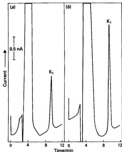
Fig. 6. Chromatograms obtained for 10 ng of phyloquinone by HPLC - EC using gaskets of (a) 0.005 mm and (b) 0.002 mm thicknesses. Mobile phase contained 95% MeOH.
