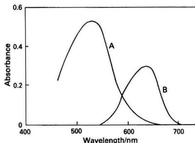
Fig. 1. Absorption spectra: A, reagent blank measured against water; and B, vanadium complex containing 5.0 µg of vanadium(V) measured against reagent blank
