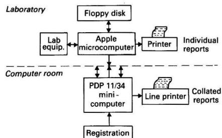
Fig. 1. Configuration of laboratory micro- and minicomputers
