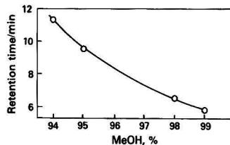
Fig. 4. Variation of retention time with percentage of methanol in the mobile phase
