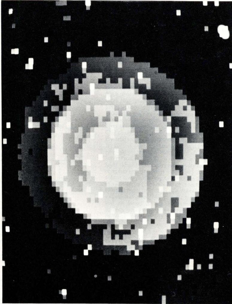
Fig. 5. Thermal wave phase image of multi-layered film
