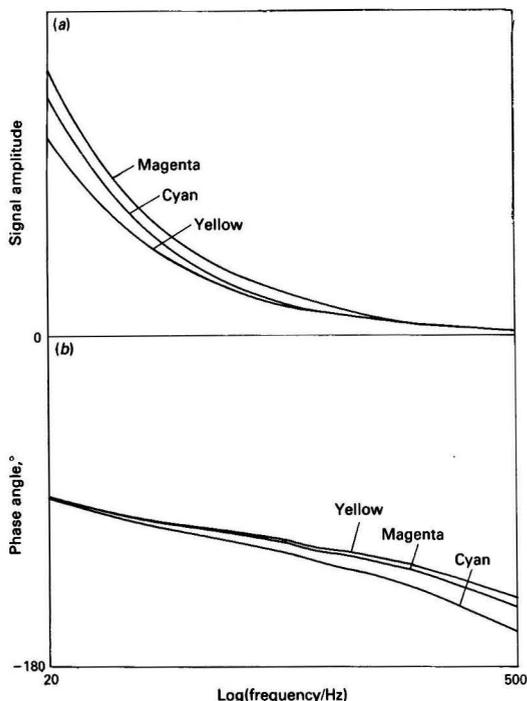
Fig. 4. Frequency response of the photoacoustic signal deriving from each of the sample zones: (a) signal amplitude; (b) signal phase
