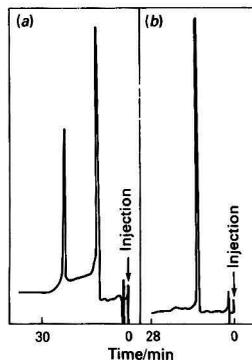
Fig. 3. Effect of variation of CTAB concentration on chromatogram obtained for sodium *N*-methyldithiocarbamate. (a) 0.001 M CTAB; (b) 0.01 M CTAB
