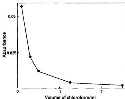
Fig. 3. Variation of the mercury absorption signal with the volume of solvent used for dissolution of the Hg - APDC complex
