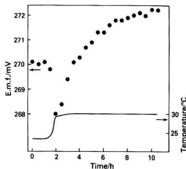
**Fig. 2.** Anomalous temperature response of aged electrode (B) in 0.01 mol l<sup>-1</sup> nitric acid medium
