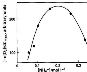
**Fig. 1.** Effect of NH<sub>4</sub><sup>+</sup> concentration on the GDH - HRP system
