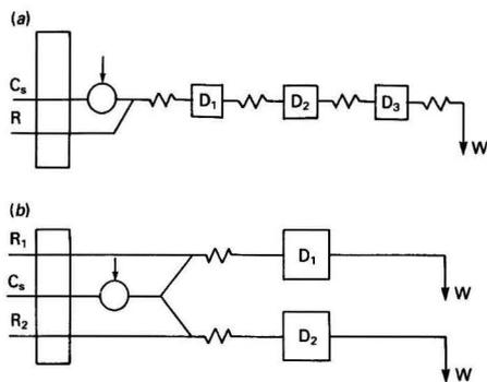
Fig. 1. Schematic diagrams of FIA manifolds for simultaneous determinations with several detectors (D). (a) In series configuration; and (b) parallel configuration with splitting up of the sample channel.  $C_s$ , Sample;  $R_1$  and  $R_2$ , reagents; and  $W$ , waste
