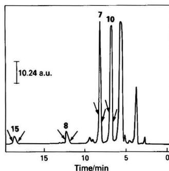
Fig. 4. Preparative HPLC of the 10th fraction from the acetone - ethanol extraction. Column: S5 ODS, 245 × 10 mm i.d. with a 50 × 10 mm i.d. pre-column. Injection: 250  $\mu$ l. Solvent: methanol - dichloromethane (80 + 20), 4 ml min<sup>-1</sup>, room temperature. Detector: 230 nm. Numbering of compounds as in Table 1
