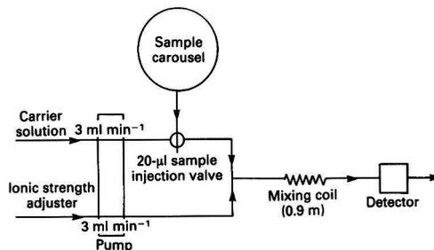
Fig. 1. Flow injection manifold
