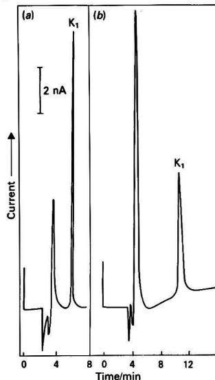
Fig. 5. Chromatograms obtained for 61 ng of phyloquinone in mobile phases containing (a) 99% MeOH - 0.05 M acetate buffer solution (pH 3.0); and (b) 95% MeOH - 0.05 M acetate buffer solution (pH 3.0)
