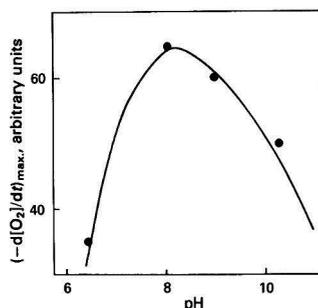
Fig. 6. Effect of pH on the lipase hydrolysis of triglycerides (by the external hydrolysis procedure)
