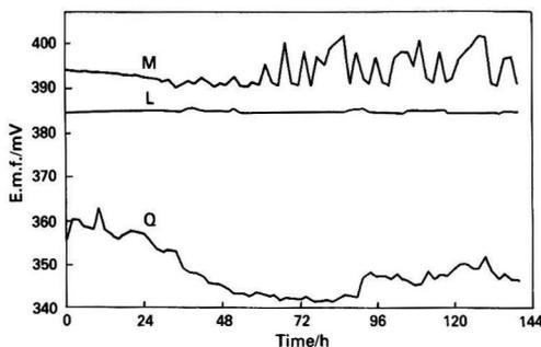
**Fig. 1.** Change of e.m.f. with time during seventh week of operation in 0.01 mol l<sup>-1</sup> nitric acid for electrodes with (L) ceramic-frit, (M) ground-glass sleeve and (Q) silicone-rubber sleeve liquid junctions
