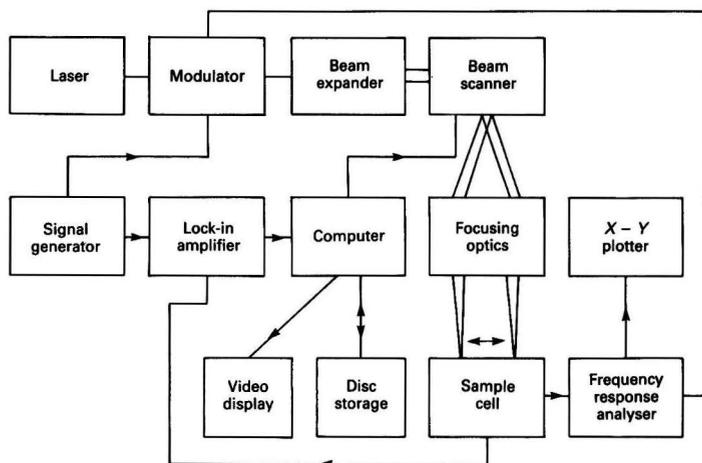
Fig. 1. Schematic diagram of thermal wave imaging apparatus
