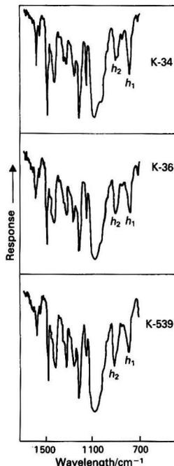
Fig. 1. IR spectra of representative nonylphenol - ethylene oxide condensates
