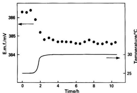
**Fig. 2.** Effect of temperature on the mercury - mercury(I) sulphate electrode in nitric acid solution
