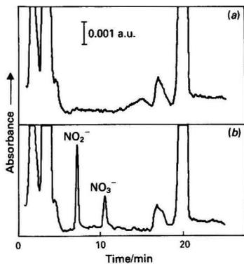
Fig. 1. Chromatogram of a sample of roast beef (a) before and (b) after spiking with  $200 \text{ mg kg}^{-1}$  of  $\text{NaNO}_2$  and  $500 \text{ mg kg}^{-1}$  of  $\text{KNO}_3$ , respectively
