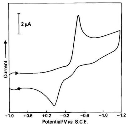
Fig. 1. Cyclic voltammogram of 10<sup>-4</sup> M phylloquinone in 95% MeOH - 0.05 M acetate buffer solution (pH 3.0) using a planar glassy-carbon electrode. Initial potential, +1.0 V; and scan rate, 20 mV s<sup>-1</sup>.
