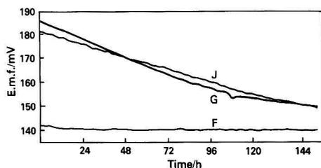
Fig. 3. Changes of e.m.f. with time during first week of test for quinhydrone - acetate (G) and quinhydrone - phthalate (J) electrodes and during eleventh week of test for quinhydrone - acetate electrode (F)
