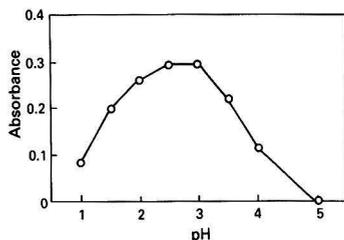
Fig. 2. Effect of pH on the formation of vanadium(V) complex. Absorbance measured at 640 nm against reagent blank
