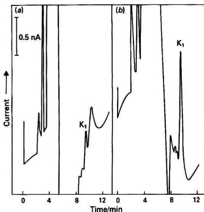
Fig. 7. Chromatograms obtained by HPLC - EC of (a) extract from 10 ml of control plasma; and (b) extract from 10 ml of plasma spiked with 0.8 ng ml<sup>-1</sup> of phyloquinone. Plasma extracts were dissolved in 70  $\mu$ l of mobile phase and 50  $\mu$ l were injected
