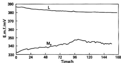
**Fig. 3.** Change of e.m.f. during the first week of the test for (M<sub>s</sub>) sealed and (L) ceramic-frit electrodes
