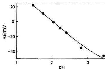
Fig. 1. Effect of pH on quinhydrone reference electrode with 0.01 mol l<sup>-1</sup> nitric acid filling solution. The solid line shows the calculated change in liquid junction potential
