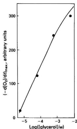
Fig. 4. Semilogarithmic plot of the calibration graph for the determination of glycerol in standard aqueous samples
