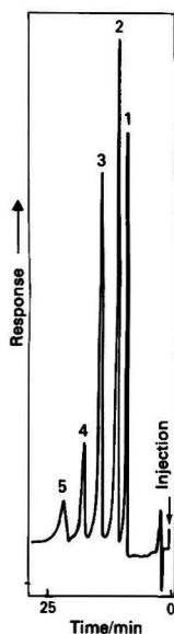
Fig. 6. Reversed-phase micellar partition chromatogram of dithiocarbamates. Solutes: 1, sodium *N*-methylthiocarbamate; 2, sodium *N,N*-dimethylthiocarbamate; (3) ammonium tetramethylenedithiocarbamate; (4) sodium *N,N*-diethylthiocarbamate; and (5) disodium ethylenebisdithiocarbamate. Conditions: column, 300 × 3.9 mm; packing, 10 μm μ-Bondapak CN; eluent, 0.0125 M CTAB (pH 6.8), methanol - water (30 + 70); temperature, 30 °C; detector, UV photometer, 253 nm, 0.01 a.u.f.s.
