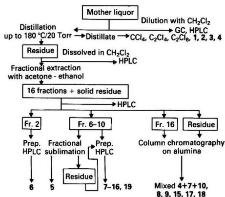
Fig. 1. Hex-waste: separation scheme for the mother liquor after crystallisation of hexachlorobenzene. Compounds numbered as in Table 1
