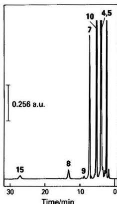
Fig. 2. HPLC of the 10th fraction from the acetone - ethanol extraction. Column: S5 ODS, 150 × 4.6 mm i.d. with a 50 × 4.6 mm i.d. pre-column. Injection: 20  $\mu$ l. Solvent: 100% methanol, 1 ml min<sup>-1</sup>, room temperature. Detector: 230 nm. Numbering of identified compounds as in Table 1
