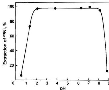
Fig. 2. Effect of pH on extraction of <sup>63</sup>Ni added to plant digests. Shaking time, 30 min. <sup>63</sup>Ni activity and counting procedure as in Fig. 1
