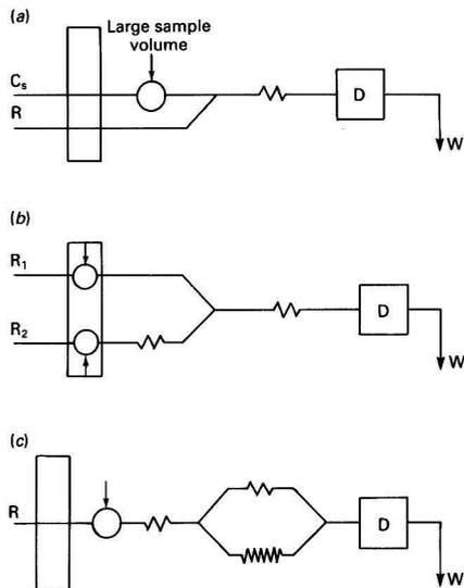
Fig. 2. Schematic diagrams of FIA manifolds for simultaneous determinations with a single detector. Several peaks are obtained for each volume injected. (a) Based on the establishment of a concentration gradient; (b) with simultaneous double injection and an asymmetric merging configuration; and (c) based on the splitting up of the sample channel into two reactors, which merge in front of the detector
