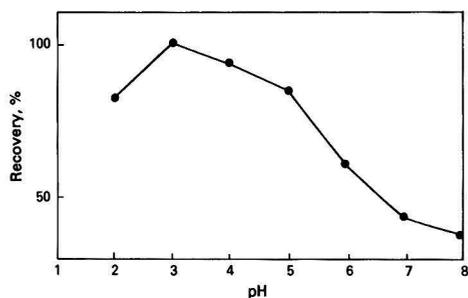
**Fig. 1.** Effect of pH on the efficiency of extraction of mercury from sea water
