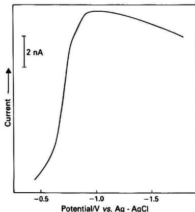
Fig. 3. Hydrodynamic voltammogram for phyloquinone in 99% MeOH - 0.05 M acetate buffer solution (pH 3.0)
