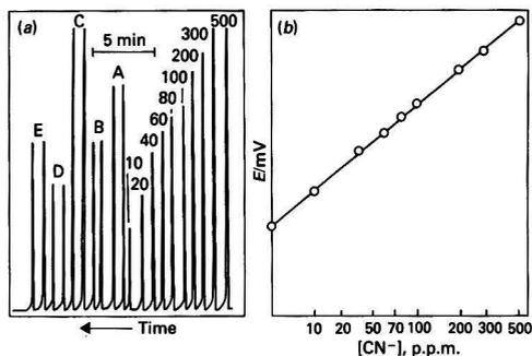
Fig. 3. Typical detector response and corresponding calibration. (a) Reading from right to left the first 10 peaks are standard solutions. The cyanide concentration (in p.p.m.) is given by the number above each. (b) Calibration graph corresponding to standards described in (a)
