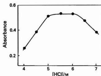
Fig. 2. Effect of hydrochloric acid concentration on absorbance of the complex at 310 nm, with  $0.13 \mu\text{g ml}^{-1}$  of gallium(III). Reference, reagent blank
