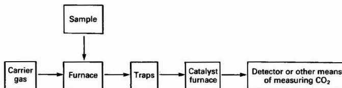
Fig. 1. Schematic diagram of the combustion process. Types of furnaces: induction; resistance; tube-type. Types of traps: dust to remove particulates (metal oxides); MnO<sub>2</sub>, to remove sulphur oxides; halogens and nitrogen oxides; sulphuric acid, to remove water vapour; and copper(I) oxide to reduce nitrogen oxides to N<sub>2</sub>
