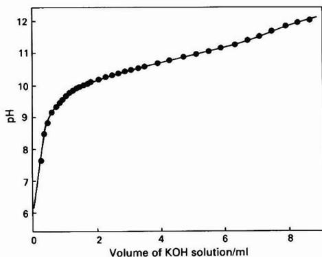
Fig. 2. Potentiometric titration curve for leucoquinizarin using a glass electrode
