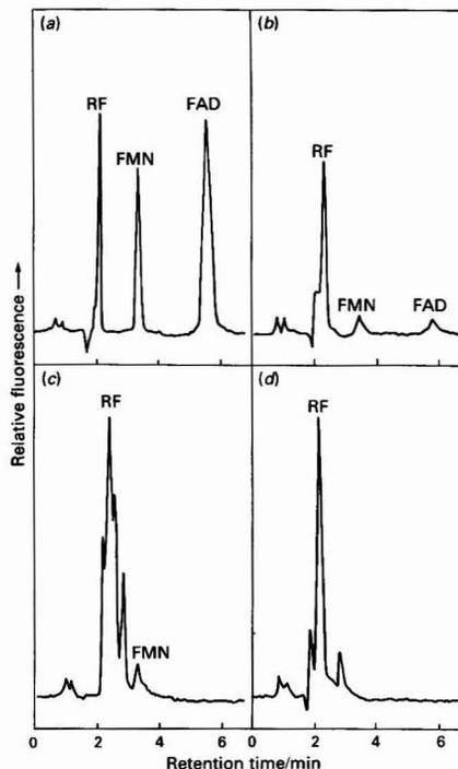
**Fig. 2.** Chromatograms of the B<sub>2</sub> vitamins in (a) standard solution; (b) sample solution treated with TCA only; (c) sample solution hydrolysed with acid; and (d) sample solution hydrolysed with enzymes. Sample: plankton body fluid
