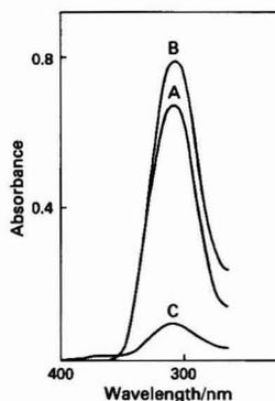
Fig. 1. Absorption spectra of: A,  $2.0 \times 10^{-5}$  M TPPP in ethanol; B,  $\text{TPPP} + \text{GaCl}_4^-$  complex extracted with 5 ml of isopentyl acetate obtained in 50 ml of aqueous solution with a Ga(III) concentration of  $2.8 \times 10^{-6}$  M, a TPPP concentration of  $4 \times 10^{-5}$  M and 6 M hydrochloric acid; and C, TPPP in isopentyl acetate
