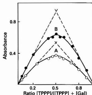
Fig. 4. Stoichiometry of gallium - TPPP complex determined by the continuous variations method. Concentration of gallium(III) plus TPPP: A,  $7 \times 10^{-6}$  M; and B,  $1 \times 10^{-5}$  M
