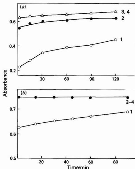
Fig. 1. (a) Influence of irradiation times and stability of the samples after irradiation. [Cu] =  $2 \times 10^{-5}$  M; [(*E*)-TAPH] =  $8 \times 10^{-5}$  M;  $\lambda$  = 427 nm; pH = 10.25. Irradiation time: 1, 0; 2, 15; 3, 30; and 4, 45 min. (b) Influence of heating times and stability of the samples after heating. Irradiation time, 30 min;  $\lambda$  = 427 nm. Heating time: 1, 0; 2, 15; 3, 30; and 4, 45 min
