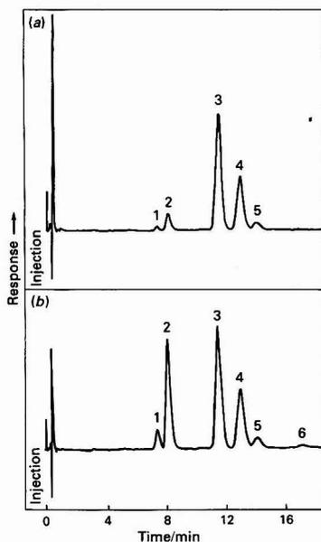
Fig. 2. Chromatograms of the nitration products of toluene with 65 + 35 V/V water - methanol as the mobile phase and an eluent flow-rate of 1.0 ml min<sup>-1</sup>. Detector, 254 nm UV, 0.01 a.u.f.s. Peaks: 1 and 2, unknowns; 3, *o*-nitrotoluene; 4, *p*-nitrotoluene; 5, *m*-nitrotoluene; and 6, toluene. Total reaction times for nitration are (a) 1.5 h and (b) 2.5 h.
