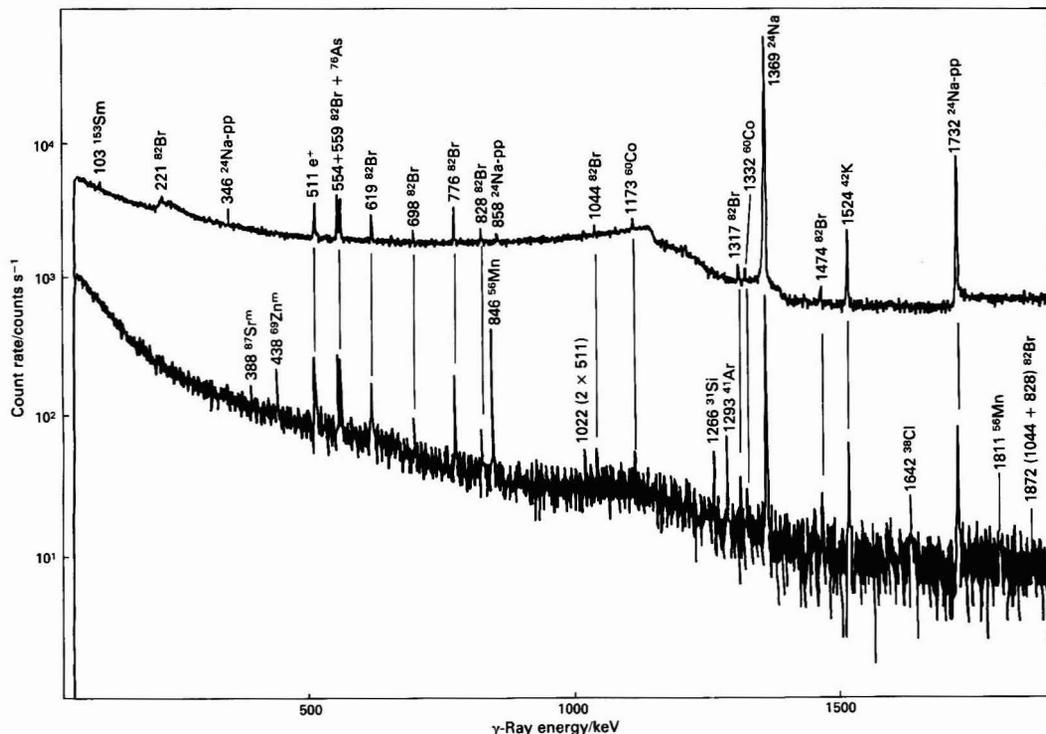
Fig. 1.  $\gamma$ -Ray spectrum of NBS SRM-1566 (oyster tissue) for brief irradiation. Upper spectrum: activation with total neutron spectrum,  $t_i = 1$  h;  $t_w = 6$  d; and  $t_c = 3600$  s. Lower spectrum: activation with epithermal neutrons,  $t_i = 1$  h;  $t_w = 2$  h; and  $t_c = 3600$  s ( $t_i =$  irradiation time;  $t_w =$  waiting time and  $t_c =$  counting time).  $^{24}\text{Na-p-p} = ^{24}\text{Na}$  gamma-ray pair-peak
