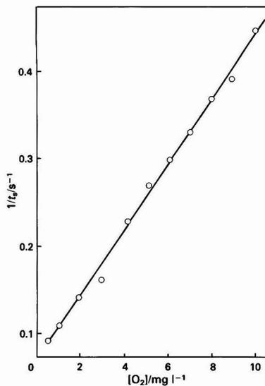
Fig. 1. Variation of the inverse of the stripping time ( $1/t_s$ ) in  $\text{s}^{-1}$  with concentration of oxygen ( $\text{mg l}^{-1}$   $\text{O}_2$ ) added to an acidic solution (pH 2) containing 250 p.p.b. of  $\text{Cd}^{2+}$ . Electrolysis time, 120 s; and applied deposition potential,  $-0.95$  V
