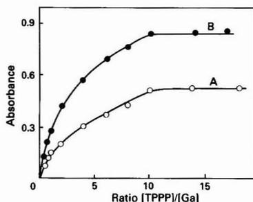
Fig. 3. Effect of reagent concentration on the absorbance of the complex. Gallium(III) concentration: A, 0.13; and B,  $0.21 \mu\text{g ml}^{-1}$
