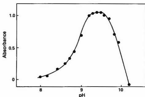
**Fig. 3.** Absorbance versus pH graph for the magnesium - leucoquinizarin chelate at 562 nm;  $C_{\text{Mg}} = 4$  p.p.m.;  $C_{\text{R}} = 5.0$  ml of 0.05% leucoquinizarin in ethanol
