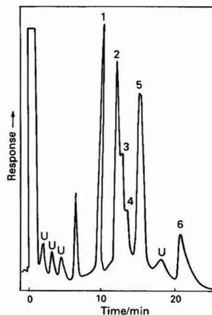
Fig. 3. Ion chromatogram of volatile amines detected in soil. 1, Methylamine; 2, dimethylamine; 3, ethylamine; 4, trimethylamine; 5, diethylamine; 6, triethylamine; and U, unknown
