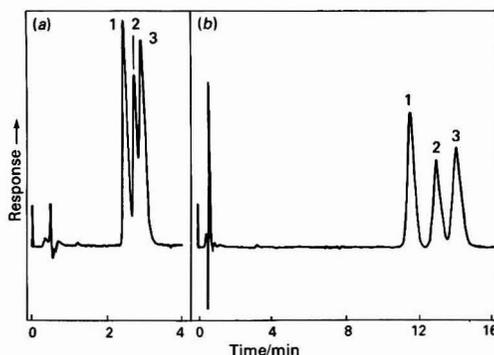
Fig. 1. Chromatograms of a standard solution of isomeric nitrotoluenes. Detector, 254 nm UV, 0.01 a.u.f.s. Peaks: 1, *o*-nitrotoluene; 2, *p*-nitrotoluene; and 3, *m*-nitrotoluene. Amounts of *o*-, *p*- and *m*-isomers are in the ratio 36.6:31.3:32.1 *mm*, respectively. Mobile phases: (a) 40 + 60 V/V water - methanol and eluent flow-rate, 0.7 ml  $\text{min}^{-1}$ ; (b) 65 + 35 V/V water - methanol and eluent flow-rate, 1.0 ml  $\text{min}^{-1}$ .
