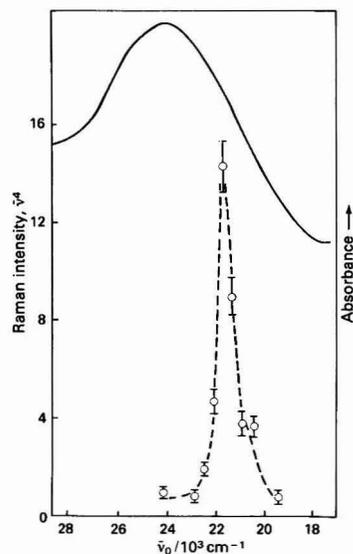
Fig. 3. Absorption spectrum of TNT in  $0.8\text{ M}$  sodium sulphite solution, and the resonance Raman excitation profile of the  $1304\text{ cm}^{-1}$  band
