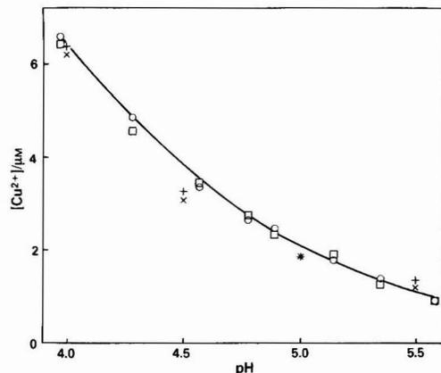
Fig. 2. Variation of  $[Cu^{2+}]$  with pH in solution 12.  $\circ$ , ISE;  $\square$ , IEE;  $+$ , GEOCHEM; and  $\times$ , ECCLES; for clarity, only the line between ISE points is shown
