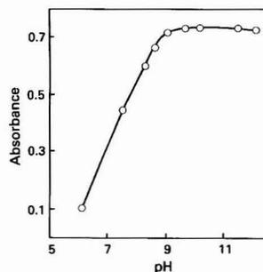
Fig. 2. Absorbance versus pH dependence for the (*Z*)-TAPH - copper complex. [Cu] =  $2 \times 10^{-5}$  M; [(*Z*)-TAPH] =  $8 \times 10^{-5}$  M;  $\lambda$  = 435 nm; and pH = 10.25
