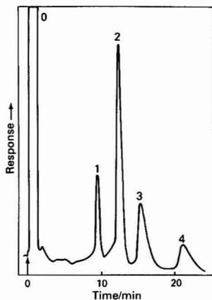
Fig. 2. Ion chromatogram of alkylamines (20  $\mu\text{g}$  of each). 0, Solvent; 1, diethanolamine; 2, dimethylamine; 3, diethylamine; and 4, triethylamine
