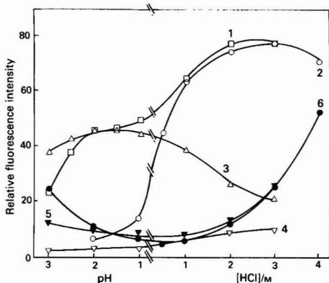
Fig. 3. Effect of hydrochloric acid concentration and pH on the relative fluorescence intensity of hafnium and zirconium complexes of 3,7-dihydroxyflavone. Graphs: 1 and 2, hafnium complex ( $2.5 \times 10^{-7}$  M Hf); 3 and 4, zirconium complex ( $2.5 \times 10^{-7}$  M Zr); 5 and 6, reagent ( $8.0 \times 10^{-5}$  M) using sulphate concentrations of 1, 3 and 5, 0.02 M and 2, 4 and 6, 0 M
