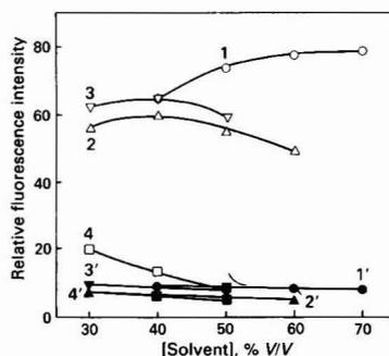
Fig. 4. Effect of the amount of solvent on the relative fluorescence intensity of zirconium - 3,7-dihydroxyflavone complex. Graphs 1–4, zirconium complex ( $4.0 \times 10^{-7}$  M Zr) using 0.2 M sulphate solution (pH 2.0) and different solvents: 1, methanol; 2, ethanol; 3, acetone; and 4, dioxane. 1'–4', Corresponding reagent ( $8.0 \times 10^{-5}$  M)
