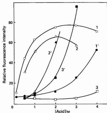
Fig. 1. Effect of acids on the relative fluorescence intensity of hafnium-3,7-dihydroxyflavone complex: 1–3 are hafnium complexes ( $2.5 \times 10^{-7}$  M Hf) in: 1, hydrochloric acid; 2, perchloric acid; and 3, sulphuric acid; 1'–3' are corresponding reagent ( $8.0 \times 10^{-5}$  M)
