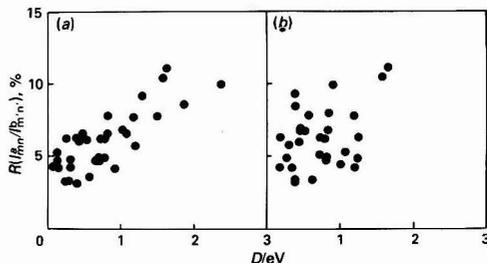
Fig. 2. Maximum relative deviations of spectral line pair (iron) intensity ratios. (a) Plotted versus  $D(E) = |hv_{mn} - hv_{m'n'}|$  ( $r = 0.80$ ) as defined in the text (side-on experiment); and (b) plotted versus  $D(E) = |E_m - E_{m'}|$  ( $r = 0.43$ ). The data set in (b) were obtained from 50 repeated measurements of Fe I line intensity ratios with an ICP as defined in the text (side-on experiment)
