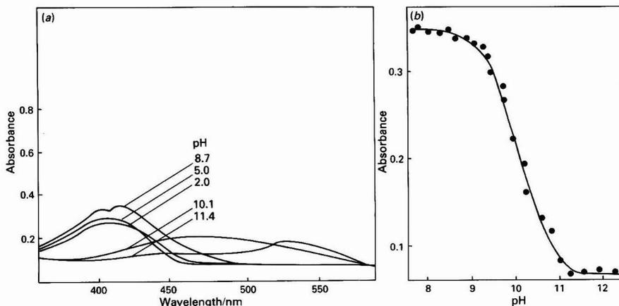
Fig. 1. Influence of pH on the absorption of the reagent. (a) Absorption spectra in 11.1% V/V ethanol at different pH values. (b) Graph of absorbance versus pH;  $C_R = 5 \times 10^{-5} \text{ M}$ ;  $\lambda = 415 \text{ nm}$
