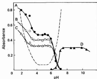
**Fig. 1.** Absorbance versus pH graph for the palladium(II) - PST complexes. Absorbances at A, 400 nm; B, 420 nm; C, 470 nm; and D, 500 nm. Dashed line, absorbance of the reagent blank at 400 nm measured against water.  $C_{\text{Pd}} = 1.8 \mu\text{g ml}^{-1}$ ;  $C_{\text{PST}} = 3 \text{ ml}$  of 0.1% solution per 25 ml; medium containing 40% DMF
