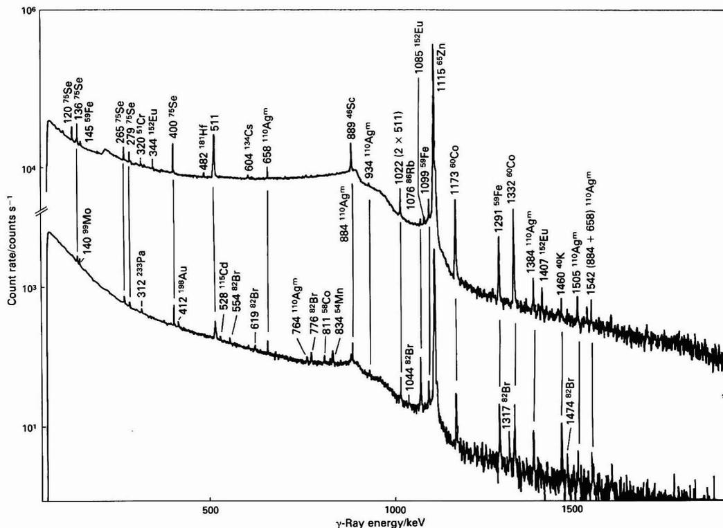
Fig. 2.  $\gamma$ -Ray spectrum of NBS SRM-1566 (oyster tissue) for prolonged irradiation. Upper spectrum: activation with total neutron spectrum,  $t_i = 48$  h;  $t_w = 50$  d; and  $t_c = 7200$  s. Lower spectrum: activation with epithermal neutrons,  $t_i = 48$  h;  $t_w = 15$  d; and  $t_c = 7200$  s.
