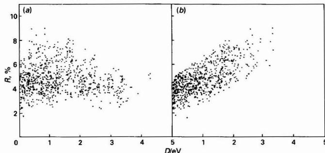
Fig. 1. Maximum relative deviation of spectral line pair (iron) intensity ratios. (a) Plotted versus  $D(E) = |E_m - E_{m'}|$  as defined in the text ( $r = -0.08$ ); and (b) plotted versus  $D(E) = |h\nu_{mn} - h\nu_{m'n'}|$  ( $r = 0.74$ ). The data in (b) were obtained from 30 repeated measurements of Fe I line intensity ratios with an ICP
