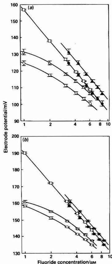
**Fig. 1.** Calibration graphs for fluoride ion-selective electrodes (a) 1 and (b) 2, using any one of three TISAB solutions, A, B and C, in the range 1–10  $\mu\text{M}$  fluoride. Nominal fluoride standard values (final concentration): A ( $\square$ ), B ( $\Delta$ ) and C ( $\circ$ ). Nominal standard fluoride values plus background fluoride: B ( $\blacktriangle$ ), C ( $\bullet$ ). Data points are means  $\pm$  2 S.E. ( $n = 3$ ). Analysis of covariance regression lines:
