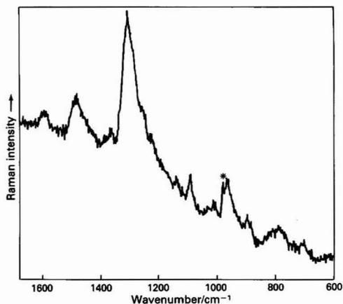
Fig. 2. Resonance Raman spectrum of  $2 \times 10^{-4}\text{ M}$  TNT in  $0.8\text{ M}$  sodium sulphite solution.  $\lambda_0 = 457.9\text{ nm}$ ; power at the sample  $\approx 100\text{ mW}$ ; scanning speed,  $1\text{ cm}^{-1}\text{ s}^{-1}$ ; spectral slit width,  $3\text{ cm}^{-1}$  at  $457.9\text{ nm}$
