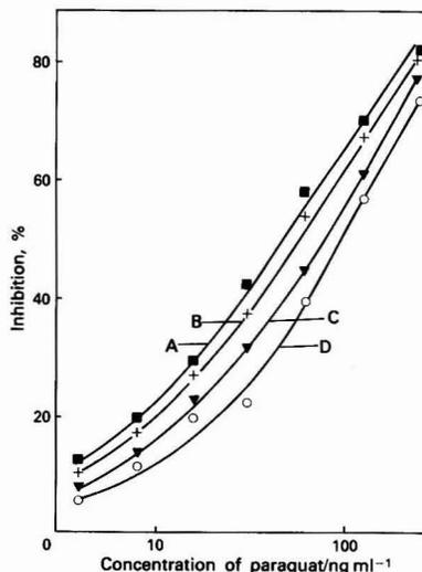
Fig. 2. Effect of sodium sulphate on the calibration graph. Plot of percentage inhibition versus paraquat concentration for solutions of incubation buffer containing: A, 0; B, 6.25; C, 25; and D, 50% of sodium sulphate
