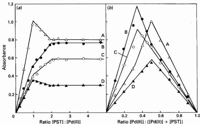
**Fig. 2.** Stoichiometry of the palladium(II) - PST complex in 40% DMF. (a) Composition determined by the molar ratio method: A, at pH 9.0 ( $C_{\text{Pd}} = 5.0 \mu\text{g ml}^{-1}$ ); B, C and D, at pH 4.5 ( $C_{\text{Pd}} = 2.9 \mu\text{g ml}^{-1}$ ). (b) Composition determined by the continuous variations method:  $C_{\text{Pd} + \text{PST}} = 1.09 \times 10^{-4} \text{ M}$ . A, at pH 9.0; B, C and D, at pH 4.5. Absorbances at A, 500 nm; B, 400 nm; C, 420 nm; and D, 470 nm
