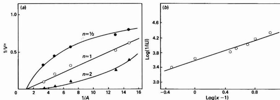
Fig. 4. Determination of the composition of the magnesium - leucoquinizarin chelate. (a) Asmus method; and (b) modified Holme and Langmyhr method. Conditions: pH 9.5 and  $\lambda = 562$  nm.  $A =$  absorbance;  $L =$  free ligand concentration;  $V =$  volume of reagent stock solution taken;  $X = A_{max}/A$ ;  $n =$  ratio of ligand to metal ion in the complex
