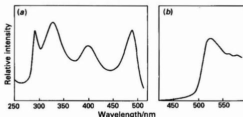
Fig. 1. (a) Excitation ( $\lambda_{em.} = 526$  nm) and (b) emission ( $\lambda_{em.} = 328$  nm) spectra of FMN in water
