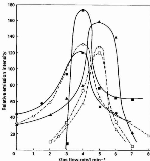
Fig. 1. Relative emission intensities with varying gas flow-rates for the Allen screw and rod techniques. Conditions:  $7.5 \mu\text{l}$  of 5 p.p.m. of Sb for both techniques; emission wavelength, 480 nm; slit width, 0.9 mm for Allen screw technique and 1.05 mm for rod method. Graphs: ■,  $\text{H}_2$ ; ●, air; ▲,  $\text{N}_2$ , Allen screw technique; and □,  $\text{H}_2$ ; ○, air; and △,  $\text{N}_2$ , rod technique
