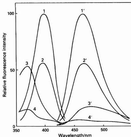
Fig. 2. Fluorescence spectra of hafnium and zirconium complexes of 3,7-dihydroxyflavone: 1–4 are excitation spectra of: 1, hafnium complex; 2, zirconium complex; 3 and 4, reagent in 1 and 3, 3 M hydrochloric acid; and 2 and 4, 0.02 M sulphate solution (pH 2.0); 1'–4' are corresponding emission spectra
