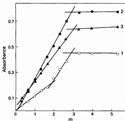
Fig. 3. Molar ratio method to study the variation of the stoichiometry of the (*E*)-TAPH-copper complex with time.  $[Cu] = 3 \times 10^{-5} M$ ;  $\lambda = 427 nm$ ; pH = 10.25; and reaction carried out in darkness. Formation time: 1, 0; 2, 3; and 3, 24 h
