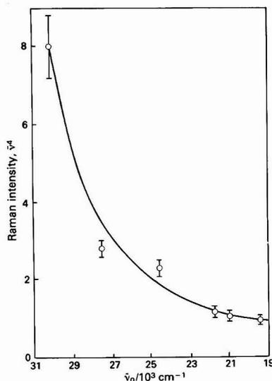
Fig. 1. Pre-resonance Raman excitation profile of the  $1358\text{ cm}^{-1}$  band of TNT in acetone solution
