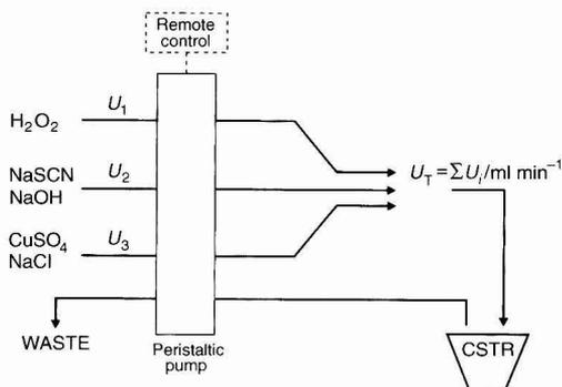
Fig. 1 Reactant and product flow across the peristaltic pump. For details, set text.
