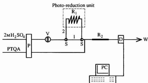
Fig. 1 Schematic representation of FI manifold employed for the simultaneous determination of Se<sup>IV</sup> and Se<sup>VI</sup>. P, Pump; V, valve; S, selector valve; R<sub>1</sub>, photoreduction coil; R<sub>2</sub>, single bead string reactor (SBSR); D, detector; W, waste; and PC, personal computer.
