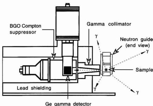
Fig. 1 Side view of the CNPGAA spectrometer in the NIST Cold Neutron Research Facility.
