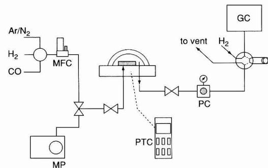
**Fig. 1** Schematic diagram of the DRIFT-GC apparatus. MP = mechanical pump; MFC = mass flow controller; PTC = programmable temperature controller; PC = pressure controller; GC = gas chromatograph equipped with methanizer and flame ionization detector. Solid line, gas lines; broken line, electrical wiring (PTC + heater).
