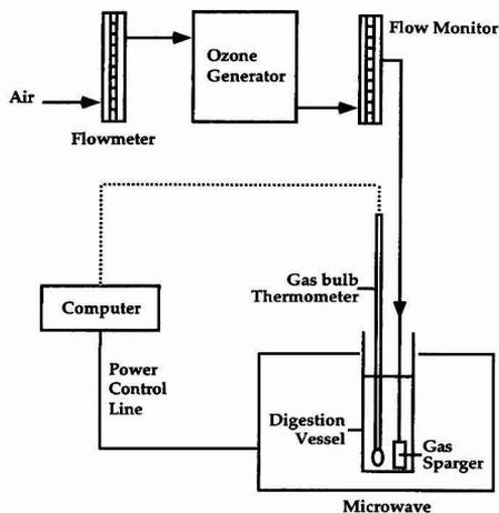
Fig. 1 Ozone apparatus set-up.
