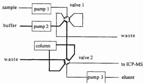
Fig. 1 Schematic diagram of matrix-analyte separation and preconcentration system. This figure shows the flow path of the system in column wash step.
