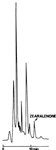
Figure 1. Chromatogram of mixed feed containing 11 \mu\text{g} zearalenone/kg: column, Spherisorb ODS 5 \mu\text{m} ; mobile phase, acetonitrile-0.1% orthophosphoric acid (50 + 50); flow rate, 1 mL/min; fluorescence detector, excitation 274 nm, emission 440 nm.
