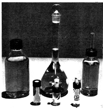
Figure 1. Test containers. Front row (l-r): 4 mL small vial, 0.3 and 1.0 mL conical vials. Back row (l-r): 3 oz prescription bottle, 100 mL volumetric flask, and 25 mL multivial (tested with the glass seal tube removed and closed with the vial cap).
