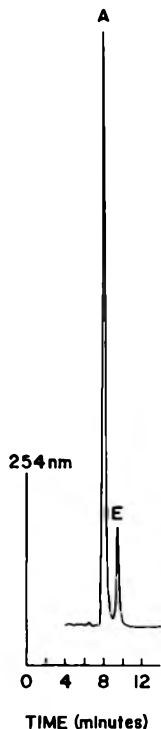
Figure 1. Chromatogram showing separation of arprinocid (A), 12 \mu\text{g}/\text{mL} ; and ethopabate (E), 2 \mu\text{g}/\text{mL} under conditions of method.
