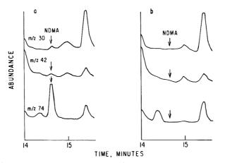
Figure 3. GC-MS of 2.8 ppb (71 ng) NDMA in extract from mineral oil distillation of malt before (a) and after (b) UV photolysis.
