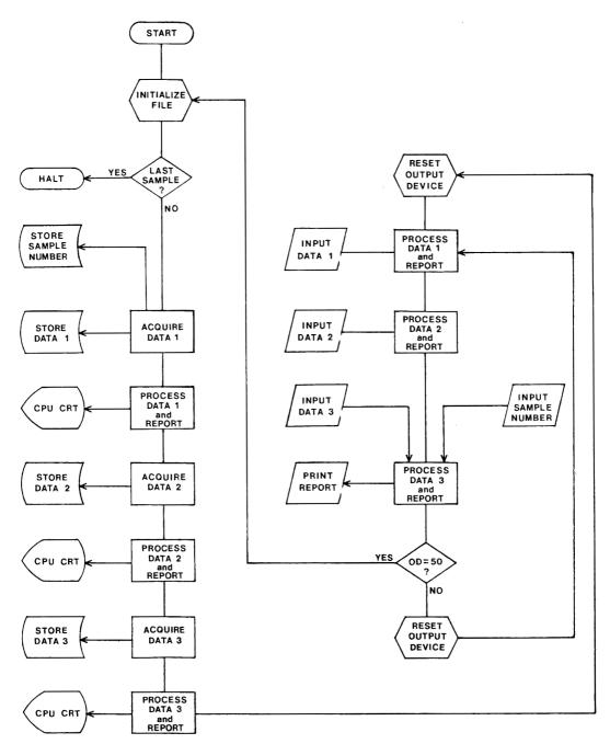
Figure 5. Flow chart of procedure to transfer abbreviated-statistical reports of triplicate analyses of sample to any 2 output devices.
