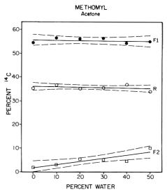
Figure 4. Percentages of carbon-14 in various fractions after extracting <sup>14</sup>C-methomyl-treated radishes, using water-acetone mixtures (see Fig. 1 for description of terms).
