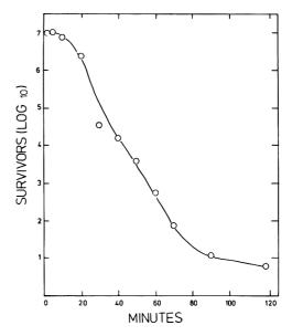
Figure 3. Effectiveness of 2% glutaraldehyde in reducing viable count on uncoated Tyvek 1073B inoculated with *B. subtilis* spores.
