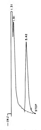
Figure 6. Chromatogram of 0 ppb (---) and 50 ppb difenzoquat in tap water.
