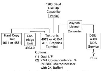
Figure 3. Configuration of communication equipment to IBM computer.
