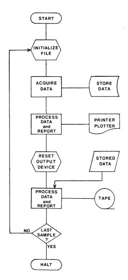
Figure 3. Flow chart of procedure for transfer to digital cartridge of duplicate reports for series of samples.
