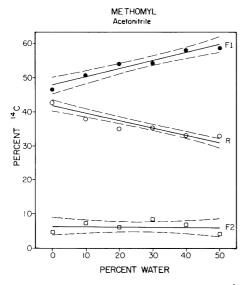
Figure 5. Percentages of carbon-14 in various fractions after extracting <sup>14</sup>C-methomyl-treated radishes, using water-acetonitrile mixtures (see Fig. 1 for description of terms).
