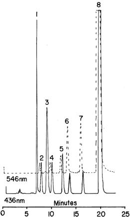
Figure 3. HPLC chromatogram of test solution of FD&C Red No. 3 (peak 8). 1 = Y-7; 2 = 4-Iodo and 4,5-Diiodo; 3 = 2-Iodo; 4 = 2,5-Diiodo; 5 = 2,7-Diiodo; 6 = 2,4,5-Triiodo; 7 = 2,4,7-Triiodo. Abbreviations are defined under *Reagents*, (c) *Stock solutions for calibrations*.
