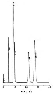
Figure 1. Typical SP 4000 chromatogram recorded by printer-plotter of solution containing (in order of elution) 4.91 ng parathion, 9.75 ng dieldrin, 1.85 ng endrin, 8.35 ng methoxychlor, and 7.4 ng mirex chromatographed on 5% OV-101 liquid phase on Chromosorb W(HP) with electron capture detection.
