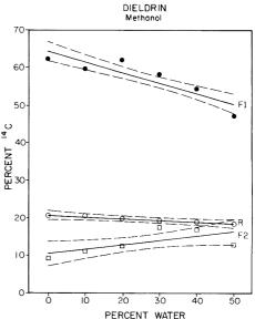
Figure 3. Percentages of carbon-14 in various fractions after extracting <sup>14</sup>C-dieldrin-treated radishes, using water-methanol mixtures (see Fig. 1 for description of terms).
