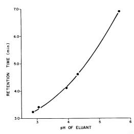
Figure 5. Effect of variation of eluant pH on retention time of difenzoquat.
