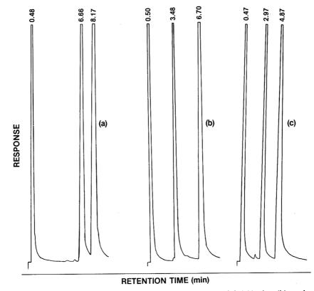
Figure 1. Typical chromatograms: (a) mephobarbital, 8.17 min; thiamylal, 6.66 min. (b) amobarbital, 3.48 min; thiamylal, 6.70 min. (c) phenobarbital (240°C), 4.87 min; thiamylal, 2.97 min.
