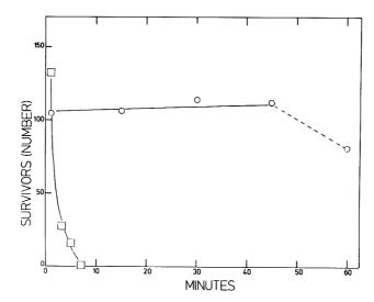
Figure 5. Comparison of polyethylene film (O) with uncoated Tyvek 1073B (△) for penetration by 2% glutaraldehyde and killing of *S. aureus*. Indirect contact method was used (see Figure 2).
