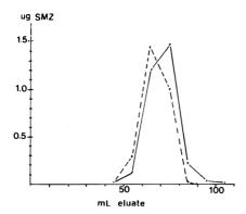
Figure 2. Typical elution profile of spiked feed after preparation of Sephadex column (—). Elution profile of Sephadex column after ca 50 samples (---).
