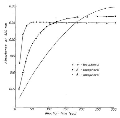
Figure 3. Reaction rate of tocopherols with ferric ion in presence of 2,2'-bypyridine (Emmerie-Engel reagent).
