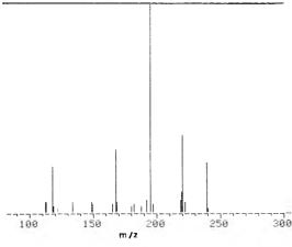
Figure 2. GC-mass spectrum of pentafluorobenzoyl derivative of dimethylamine.
