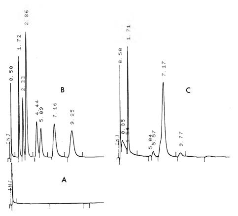
Figure 1. Gas chromatograms of (A) reagent blank, (B) amine standard solution, and (C) 1 g barley/mL. Operating conditions given in text; 5 μL injection, Ultra-Bond column, 256 attenuation. Peak identity (ng): dimethylamine, 1.72 min (25), diethylamine (25), diisopropylamine (50), di-*n*-propylamine (50), isopropylamine (50), methylamine, 7.16 min (100), and propylamine (100).
