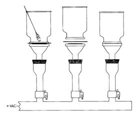
Figure 1. Three stages of direct contact procedure for testing penetration of packaging material by antimicrobial agents. Filter funnel (right) contains membrane filter inoculated with test bacteria. Funnel is raised (middle) and sample of packaging material is inserted over inoculated membrane. Funnel is replaced (left) and packaging material is swabbed with antimicrobial agent.
