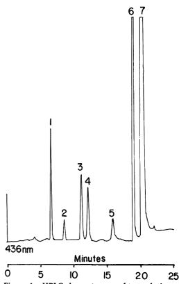
Figure 4. HPLC chromatogram of test solution of FD&C Red No. 3 (peak 7). 1 = Y-7; 2 = 4-Iodo; 3 = 2-Iodo; 4 = 4,5-Diiodo; 5 = 2,5-Diiodo; 6 = 2,7-Diiodo and 2,4,5-Triiodo; 7 = 2,4,7-Triiodo and FD&C Red No. 3. Abbreviations are defined under *Reagents*, (c) Stock solutions for calibrations.
