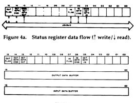
DRII-K Register Aufgements Figure 4b. Register assignments.
