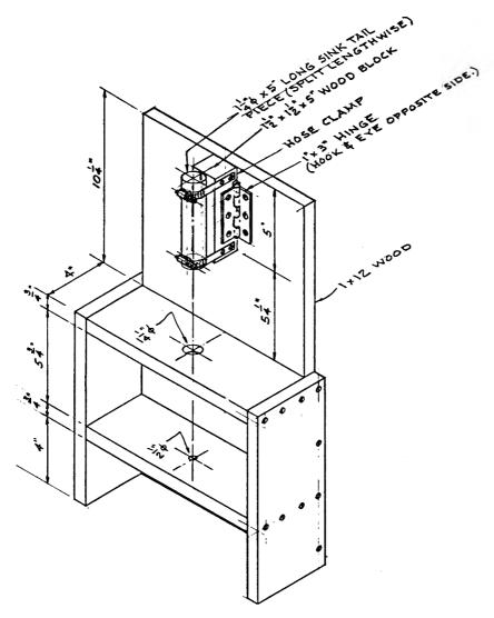
Figure 1. Pneumatic compeller.
