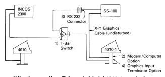
Figure 2. Hardware modifications to allow Tektronix Model 4010-1 terminal communication to Finnigan MAT SS-100 and INCOS 2300 data systems.
