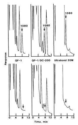
Figure 1. Gas chromatographic analysis of stomach content on 3 different colunns; lower chromatograms, control sample; upper chromatograms, 1 g sample fortified with 1 μg 1080; 1 μL injection (equivalent to 0.2 mg sample); attenuation at 64.
