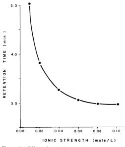
Figure 3. Effect of variation of eluant ionic strength on retention time of difenzoquat.
