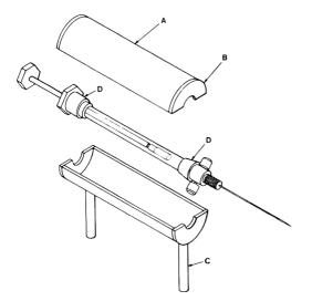
Figure 1. Metal syringe mantle, adapted for 1 mL Pressure-Lok® syringe: A, 1.5 in. id copper pipe cut lengthwise into 2 pieces; B, 0.0625 in. thick copper plate, one for each end; C, 0.25 od × 2 in. copper pipe, 2 pieces; D, rubber tubing gasket over metal end fittings of syringe.
