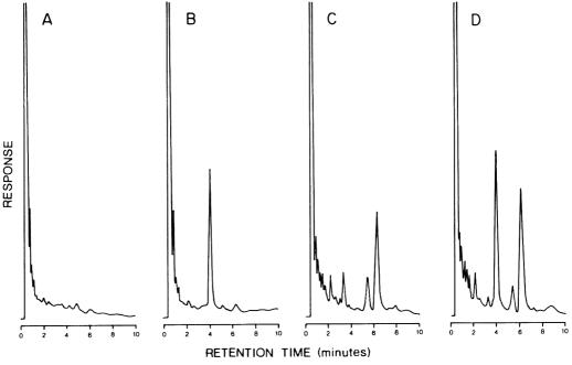
Figure 1. EC chromatograms obtained by described method (3% OV-1 at 230°C): A, reagent blank; B, CPA standard, retention time 4.03 min; C, unfortified sample of mung bean sprouts; D, sample fortified with 0.20 ppm CPA; similar chromatogram as D for "rootless" sample.
