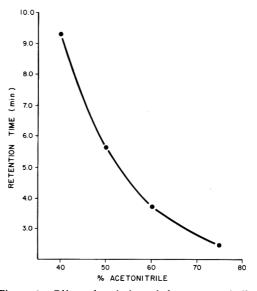
Figure 4. Effect of variation of eluant acetonitrile concentration on retention time of difenzoquat.
