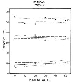
Figure 6. Percentages of carbon-14 in various fractions after extracting <sup>14</sup>C-methomyl-treated radishes, using water-methanol mixtures (see Fig. 1 for description of terms).
