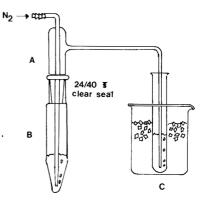
Figure 1. Diazomethane generator: A, bubbler tube with ca 1 mm id orifices; B, reaction tube with ca 20 mL volume; C, test tube receiver with ice water bath
