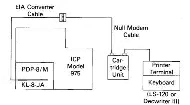
Figure 2. Hardware interface of high speed printer and data cartridge to ICAP.
