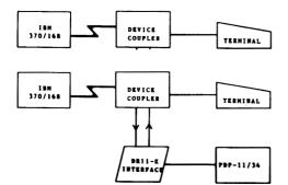
Figure 5. Device coupler operation.
