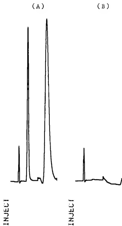
Figure 3. HPLC chromatograms of (A) feed spiked at 0.0055% carbadox and 0.0106% pyrantel tartrate and (B) the same feed unspiked.
