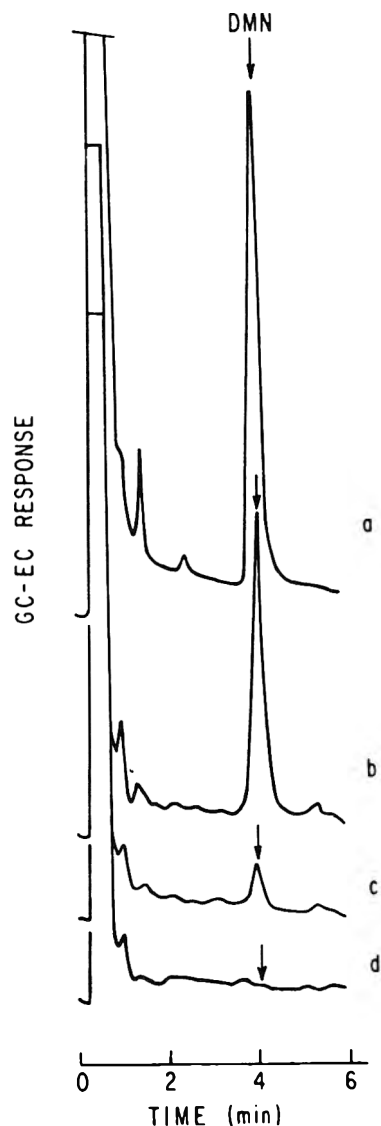
Figure 4. GC-EC chromatogram at column temperature of 140°C: (a) 0.1 ng DMN standard; (b) beer sample extract after peroxidation and cleanup steps; (c) fried cure-pumped bacon sample extract after peroxidation and cleanup steps; (d) blank.
