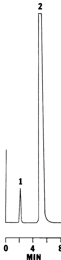
Figure 2. LC chromatogram of (1) fluorouracil and (2) flucytosine. Chromatographic conditions: column, mobile phase, flow rate, and temperature as described in method. Wavelength 266 nm; detector attenuation 0.08 AUFS; chart speed 0.5 cm/min.
