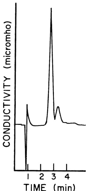
Figure 1. Typical chromatogram of cacodylic acid formulation sample. Solvent front (ca 0.8 min), cacodylic acid (ca 2.6 min), and methanearsonic acid impurity (ca 3.2 min).
