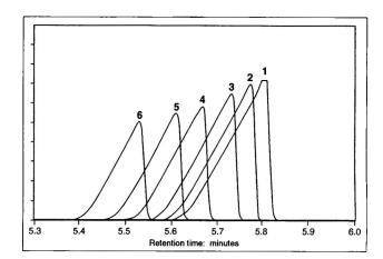
Figure 1. Split flow experiment conducted to determine the split ratio necessary to prevent integrator analog to digital (A-D) converter overload. Split flow (mL/min): 1, 100; 2, 120; 3, 140; 4, 160; 5, 180; 6, 200.
