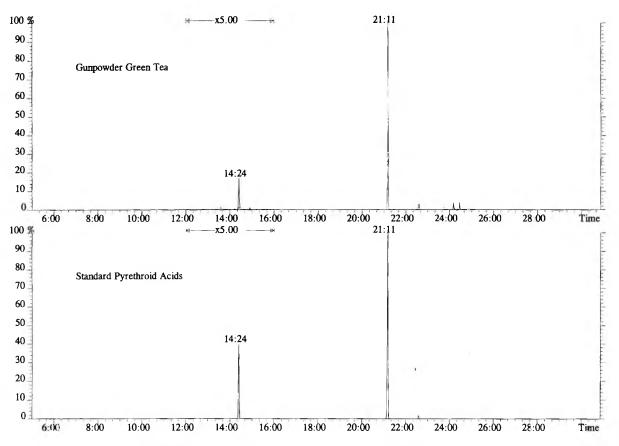
Figure 5. Comparison of GC/MS traces at *m/z* 364 of an extract of gunpowder green tea and standard hexafluoroisopropyl esters of pyrethroid acids that confirm the presence of fenvalerate (14.25 min) and 3-phenoxybenzoic acid (21.11 min) in the tea (each trace is individually normalized to its largest peak).
