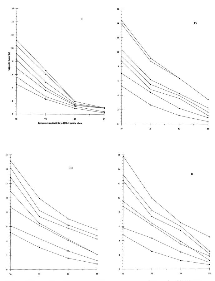
Figure 1. Effect of mobile phase composition on the elution of isocyanate derivatives on various LC stationary phases: I, Spherisorb C8; II, Spherisorb S50DS1; III, Spherisorb S50DS2; IV, Nucleosil 120 5C18; V, Partisil ODS3; and VI, Zorbax Z0DS.
