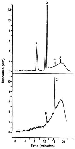
Figure 8. Chromatograms of products of periodate (top) and electrochemical (bottom) oxidation of B2. Refer to Figure 6 for explanation of product letters.
