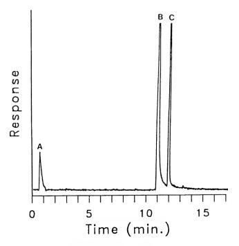
Figure 1. Chromatogram of an acetone extract of goat milk spiked with methyl paraoxon (MPO) and methyl parathion (MPT) at 5  $\mu$ g/mL: acetone, A; MPO, B; MPT, C.
