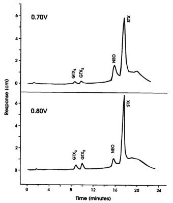
Figure 4. Verification of NEO peak by changing the oxidation potential. The 2 chromatograms were obtained at different oxidation potentials: 0.70 and 0.80 V. As the potential was increased, the peak height for nonhydroxylated toxins (STX, GTX 2/3) increased, while the peak height for NEO decreased.
