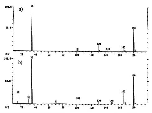
Figure 3. PICI mass spectra of 4-chloro-6-methoxyindole (a) and 6-chloro-4-methoxyindole (b).
