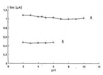
Figure 4. Dependence of limiting current on pH. (A) wave 1; (B) wave 2.
