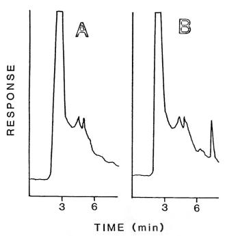
Figure 2. LC/UV chromatograms of (A) control grass hay and (B) grass hay fortified at 0.05 ppm.
