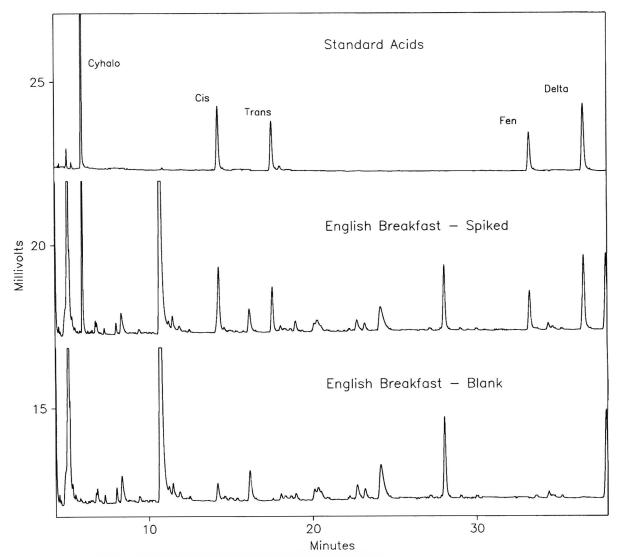
Figure 2a. Comparison of the early eluting part of the GC–ECD traces of extracts of English breakfast tea (spiked and blank) and standard pyrethroid acids (as hexafluoroisopropyl esters). Abbreviations: cyhalo, cyhalothrin acid; cis, *cis*-permethrin acid; trans, *trans*-permethrin acid; fen, fenvalerate; delta, deltamethrin.
