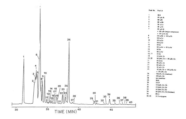
Figure 994.15.  $C_{18}$  region of the gas chromatogram of the fatty acid methyl esters from partially hydrogenated soybean oil, using 100 m  $\times$  0.25 mm fused silica capillary column coated with SP2560.
