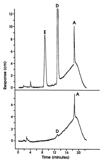
Figure 7. Chromatograms of products of periodate (top) and electrochemical (bottom) oxidation of NEO. Refer to Figure 6 for explanation of product letters.
