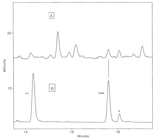
Figure 6. Comparison of a section of the GC–ECD chromatograms of (A) an extract of lapsang souchong tea and (B) standard *cis*- and *trans*-permethrin acids (as hexafluoroisopropyl esters) that show a residue of these acids in the tea (X is a reagent blank contaminant).
