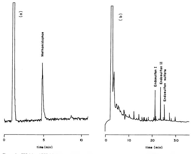
Figure 2. FPD (a) and ECD (b) chromatograms corresponding to extracts obtained for COEXPHAL sample 1 in extraction B<sub>1</sub> at 300 atm (*see* Table 3 for extraction conditions and determined pesticide levels).
