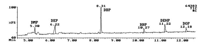
Figure 6. GC/MS chromatogram of a 20  $\mu$ g/L phthalates mix standard.
