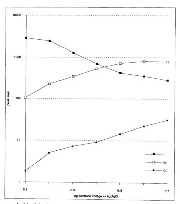
Figure 2. Relative responses of chloride, bromide, and iodide to the silver electrode at different potentials.
