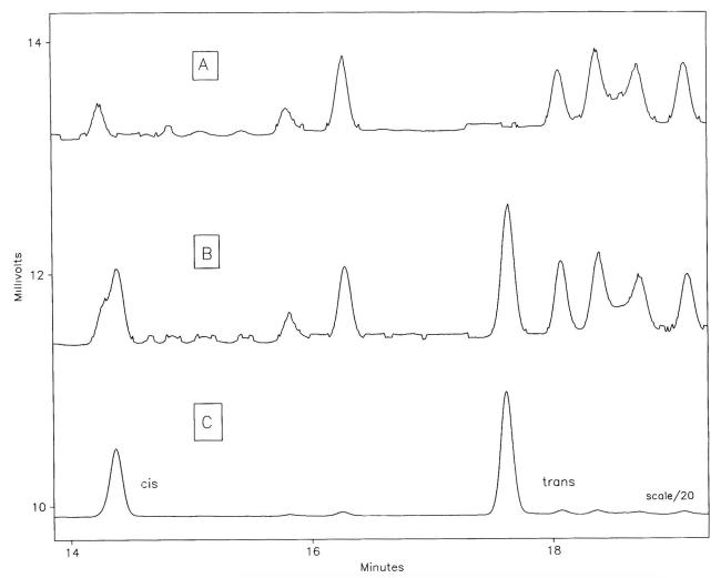
Figure 3. Comparison of a section of the GC–ECD chromatograms of extracts of orange pekoe: (A) blank, (B) spiked with permethrin glucosides at 0.05 ppm, and (C) spiked with permethrin glucosides at 1 ppm. Samples were hydrolyzed and derivatized prior to analysis.
