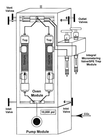
Figure 1. Schematic diagram of prototype SFE system.
