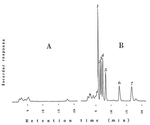
Figure 3. Chromatogram of blank (A) and spiked (10 ppb) bovine serum samples (B): (1) PABA (internal standard), (2) SDZ, (3) STZ, (4) SMT, (5) SMM, (6) SMX, and (7) SDM. Their retention times after acetonitrile extraction and fluorescamine derivatization were 5.6, 6.3, 6.7, 7.2, 8.1, 12.5, and 16.5 min, respectively.
