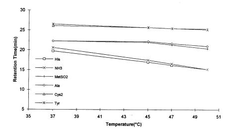
Figure 1. Effect of column temperature on separation of derivatized sulfur-containing amino acids and other amino acids: pH of eluent A, 4.95; gradient conditions, 100% A at initial time, 93% A at 17 min, 80% A at 21 min, and 60% A at 32 min (all curves linear).
