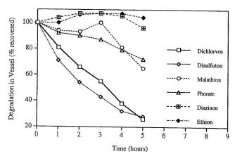
Figure 3. Degradation rates of 6 organophosphorus insecticides in potato samples kept in SFE vessels for 1–5 h at room temperature and exposed to air.
