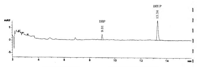
Figure 4. Liquid chromatogram of vodka sample containing DBP at 34  $\mu$ g/L and DEHP at 320  $\mu$ g/L.
