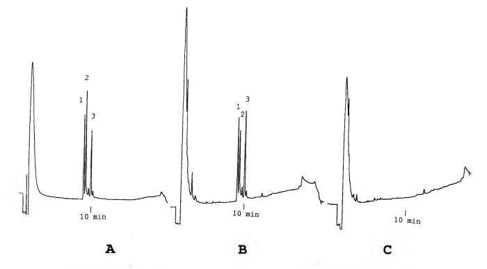
Figure 2. Chromatogram of A, a mixed standard of 1.0 ng each: 1, desethylatrazine; 2, desisopropylatrazine; and 3, atrazine. Chromatogram of B, 10 mg injection of corn extract spiked with 0.10 ppm each of the triazine compounds. Chromatogram of C, 10 mg injection of unspiked corn sample.
