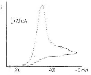
Figure 5. Cyclic voltammogram of 1 mM nitroxynil at pH 6.0 and a sweep rate of 1 V/s.
