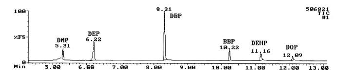
Figure 5. GC/MS chromatogram of a 500  $\mu$ g/L phthalates mix standard.
