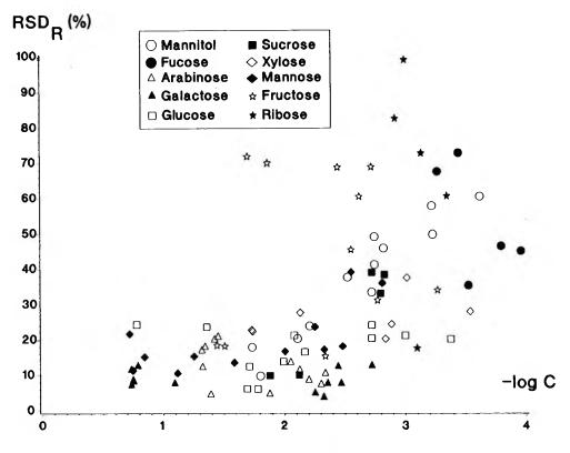
Figure 2. Precision parameters (RSD<sub>R</sub>) for carbohydrate as a function of concentration (-log C).
