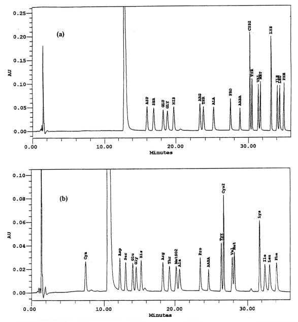
Figure 2. Chromatography of derivatized amino acid standard mixtures for (a) common amino acids (255 pmol) and (b) common and sulfur-containing amino acids (100 pmol). Separation conditions are described in *Experimental*.
