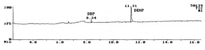
Figure 7. GC/MS chromatogram of vodka sample containing DBP at 34  $\mu$ g/L and DEHP at 320  $\mu$ g/L.
