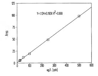
Figure 8. Standard curve of DBP by GC/MS.
