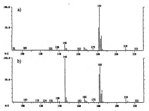
Figure 4. NICI mass spectra of 4-chloro-6-methoxyindole (a) and 6-chloro-4-methoxyindole (b).
