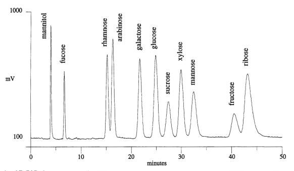
Figure 1. AE–PAD chromatogram of a mixed standard solution: mannitol, 15  $\mu$ g/mL; fucose, 15  $\mu$ g/mL; rhamnose, 35  $\mu$ g/mL; arabinose, 40  $\mu$ g/mL; galactose, 50  $\mu$ g/mL; glucose, 55  $\mu$ g/mL; sucrose, 45  $\mu$ g/mL; xylose, 55  $\mu$ g/mL; mannose 45  $\mu$ g/mL; fructose, 90  $\mu$ g/mL; and ribose, 90  $\mu$ g/mL.
