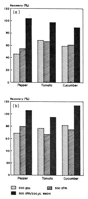
Figure 1. Methamidophos recoveries from spiked vegetable samples by SFE (dynamic mode after a 1 min static equilibrium with 15 mL of compressed CO<sub>2</sub> at 50°C and 3 pressure-modifier conditions): (a) 2.5 mg/kg spiking level and 2.5 mL extraction cartridge; (b) 0.5 mg/kg spiking level and 10 mL extraction cartridge.
