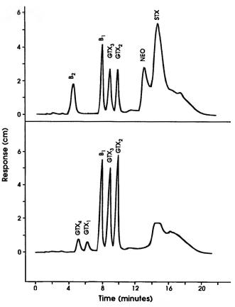
Figure 5. Typical chromatograms of mixtures of PSP standards. Oxidation parameters were pH 7 and 0.75 V. Amounts injected (ng) for top panel: B2, 90; B1, 11; GTX 3, 0.97; GTX 2, 4.0; NEO, 7.0; STX, 0.94. Amounts injected for bottom panel: GTX 4, 9.0; GTX 1, 26; B1, 11; GTX 3, 2.5; GTX 2, 7.5.
