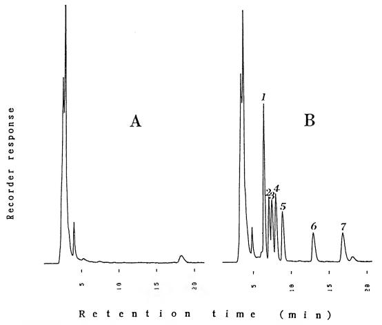
Figure 4. Chromatogram of blank (A) and spiked (10 ppb) milk samples (B): (1) PABA (internal standard), (2) SDZ, (3) STZ, (4) SMT, (5) SMM, (6) SMX, and (7) SDM. Their retention times after acetonitrile extraction and fluorescamine derivatization were 5.6, 6.3, 6.7, 7.2, 8.1, 12.5, and 16.5 min, respectively.
