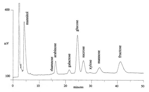
Figure 8. AE–PAD chromatogram of free carbohydrate profile of a soluble coffee containing coffee husks or parchments and cereals (sample 63).
