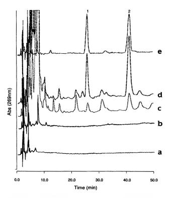
Figure 2. Analytical reversed-phase chromatograms of extracts of reagent blank (a), skim milk (b), whole milk (c), infant formula (d), and standards (e). Conditions: column, 5  $\mu$ m C<sub>18</sub> Resolve; mobile phase, methanol–isopropyl alcohol–ethylacetate–water (450 + 350 + 145 + 135); flow rate, 2.0 mL/min; detection, 269 nm (0.005 aufs; 0.002 aufs for whole milk extract). Peak 1, vitamin K<sub>1</sub> (*cis* + *trans*); peak 2, cholesteryl phenylacetate.
