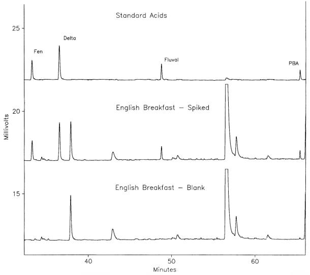
Figure 2b. Comparison of the late eluting part of the GC–ECD traces of extracts of English breakfast tea (spiked and blank) and standard pyrethroid acids (as hexafluoroisopropyl esters). Abbreviations are as defined in the caption to Figure 2a. Fluval, fluvalinate acid; PBA, 3-phenoxybenzoic acid.
