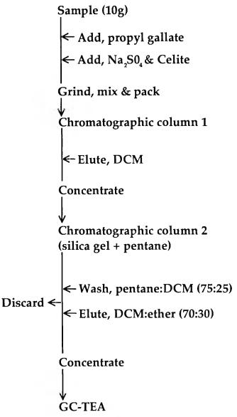
Figure 2. Flow diagram of SPE procedure.
