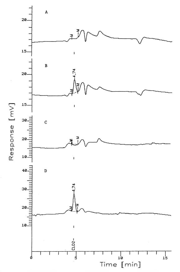
Figure 3. Chromatograms of representative rinse water samples from cut, raw green beans before (A) and after (B) fortification with 0.100 ppm chlorite and 0.086 ppm chlorate and sliced, raw carrots before (C) and after (D) fortification with 0.084 ppm chlorite and 0.078 ppm chlorate. Amperometric detection was used. Response scales are dissimilar.
