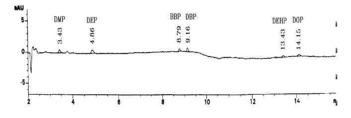
Figure 3. Liquid chromatogram of a 20  $\mu$ g/L phthalates mix standard.
