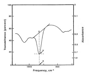
Figure 994.14. IR spectrum of partially hydrogenated canola oil methyl esters (2% solution in CS<sub>2</sub>).
