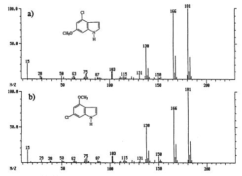
Figure 2. El mass spectra of 4-chloro-6-methoxyindole (a) and 6-chloro-4-methoxyindole (b).
