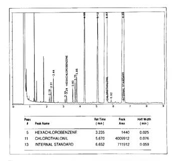
Figure 2. Typical gas chromatogram from analysis of Bravo 720.
