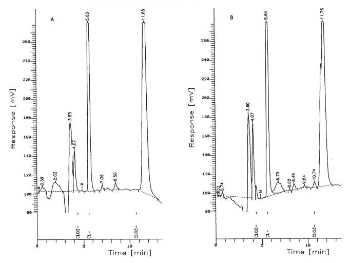
Figure 2. Chromatograms of representative rinse water samples from cut, raw green beans before (A) and after (B) fortification with 0.100 ppm chlorite and 0.086 ppm chlorate. Conductivity detection was used.
