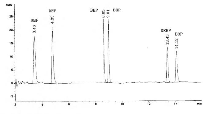
Figure 2. Liquid chromatogram of a 1.0 mg/L phthalates mix standard.
