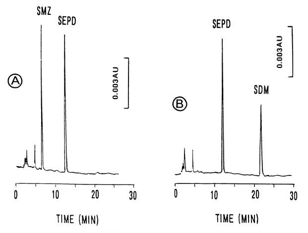
Figure 5. Chromatograms of a 25  $\mu$ L injection of extracts obtained from check sample S-1142 (A) and check sample S-1143 (B) analyzed by our LC method as part of the interlaboratory check sample testing program. S-1142 was determined to contain SMZ at 103 ng/g and S-1143 was found to contain SDM at 162 ng/g.
