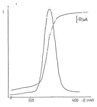
Figure 2. Typical dc wave and ac peak polarograms of 0.1 mM nitroxynil at pH 6.0.
