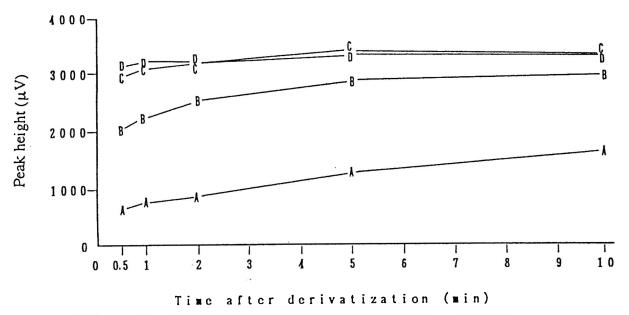
Figure 1. Stability of derivatives obtained by reacting 0.5 mL sulfamethazine (0.01  $\mu$ g/mL) with 0.1 mL fluorescamine at different concentrations (A, 0.1; B, 0.5; C, 1.0; D, 1.5 mg/mL).
