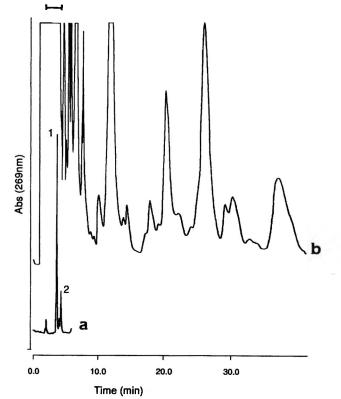
Figure 1. Semipreparative chromatogram of standards (a) and a typical infant formula (b). Conditions: column, 5  $\mu$ m silica Resolve; mobile phase, hexane-isopropyl alcohol (99.9 + 0.1); flow rate, 2.0 mL/min rising to 8.0 mL/min after fraction collection; detector, 269 nm (0.16 aufs). Peak 1, cholesteryl phenylacetate + *cis*-vitamin K<sub>1</sub>; peak 2, *trans*-vitamin K<sub>1</sub>; peak - collection window.
