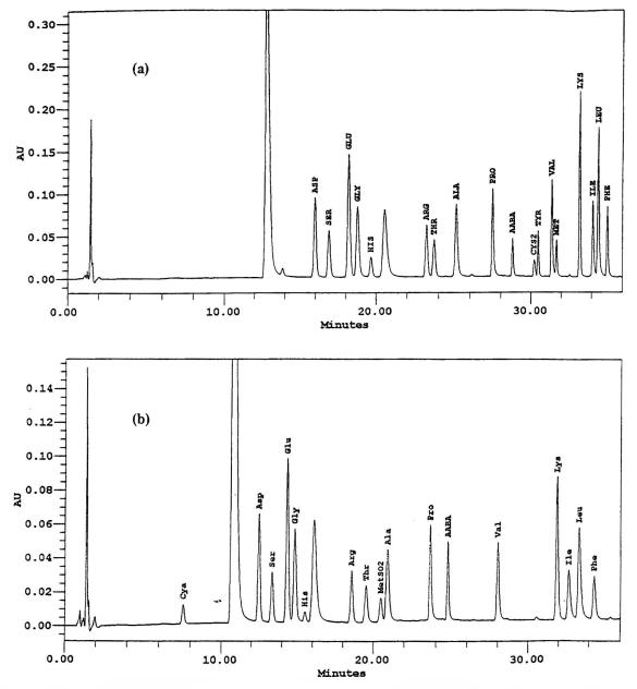
Figure 5. Chromatogram of amino acids derivatives in (a) acid hydrolyzed broiler starter sample and (b) performic acid oxidized broiler starter hydrolysate.
