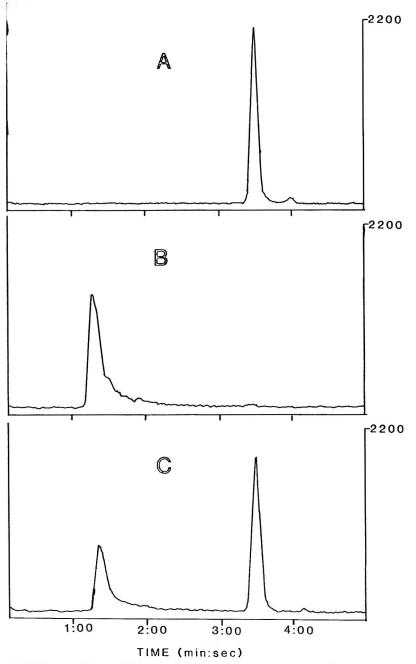
Figure 3. Chromatograms from LC/MS of (A) 5 ng hydramethylnon standard, (B) control grass hay, and (C) grass hay fortified at 0.05 ppm.
