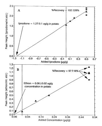
Figure 3. Results of method of standard addition for (A) iprodione and (B) ethion in potato check sample. Actual iprodione and ethion concentrations were 1.6 and 0.12  $\mu$ g/g, respectively. Legend: (I), check samples fortified with pesticides at 0.5  $\mu$ g/g before SFE, and ( $\blacktriangle$ ), fortified extracts used for calibration. Recoveries were 100% for the pesticides. The reason for the differences in experimental and expected ethion concentrations is unknown.
