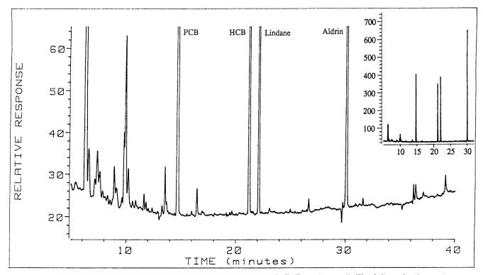
Figure 1. Typical GC–ECD chromatogram of potato extracted by SFE (Experiment 1). The full-scale chromatogram in the upper right shows the peak signals, and the larger chromatogram gives the noise levels of the potato extract, which was analyzed without additional cleanup. PCB, 0.14  $\mu$ g/g; HCB, 0.26  $\mu$ g/g; lindane, 0.37  $\mu$ g/g; aldrin internal standard, 0.36  $\mu$ g/g.
