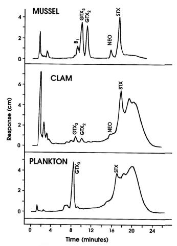
Figure 9. Chromatograms depicting separation of PSP toxins in various extracts. The mussel extract contained total PSP toxin at 25  $\mu$ g/g, and the clam extract was contaminated at 1  $\mu$ g/g (0.5 g tissue mL; dilution factor, 1/30 for both samples). Plankton chromatogram is qualitative only. Integrator attenuation was set at 8 for the mussel sample and at 5 for the clam and plankton samples.
