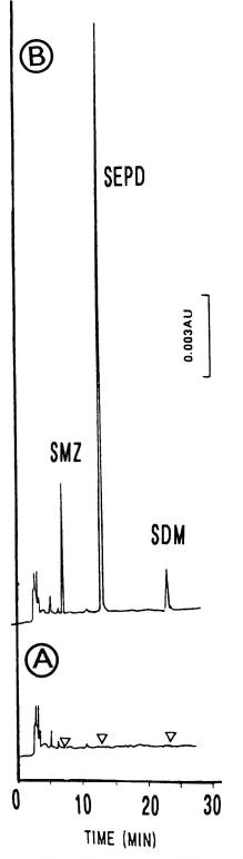
Figure 1. Typical chromatograms of a 50  $\mu$ L injection of muscle tissue extract from a control (untreated) porcine muscle (A) and a control porcine muscle fortified with SMZ and SDM at 20 ng/g tissue and 160 ng/g of the internal standard, SEPD (B).
