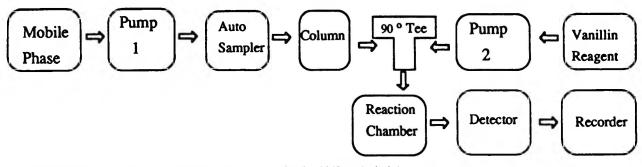
Mobile Phase = methanol/water/acetic acid 94/6/0.1 (v/v/v)
