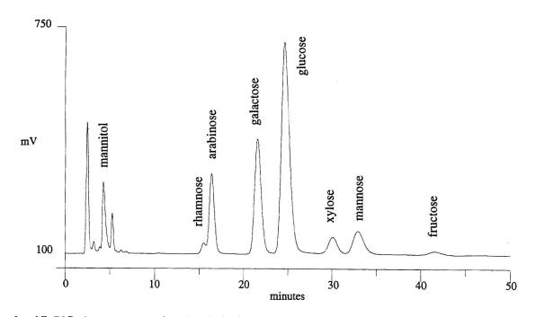
Figure 9. AE–PAD chromatogram of total carbohydrate profile of a soluble coffee containing coffee husks or parchments and cereals (sample 63).
