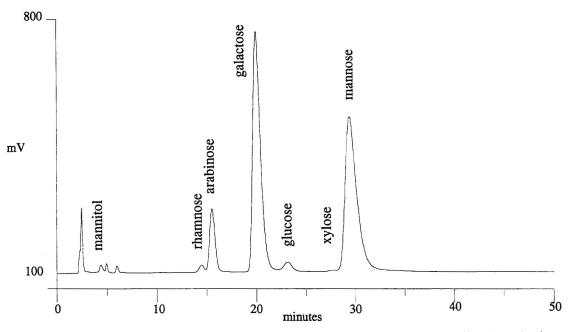
Figure 2. AE-PAD chromatogram of typical free carbohydrate profile of a pure soluble coffee (sample 1).
