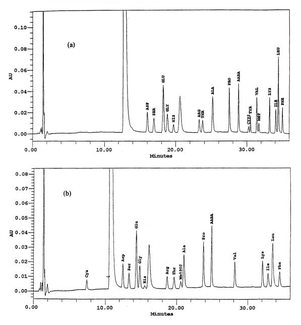
Figure 4. Chromatogram of amino acid derivatives in (a) acid hydrolyzed corn sample and (b) performic acid oxidized corn hydrolysate.
