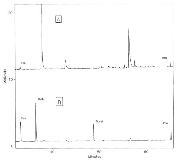
Figure 4. Comparison of a section of the GC–ECD chromatograms of (A) gunpowder green tea and (B) standard pyrethroid acids (as hexafluoroisopropyi esters) showing a residue of fenvalerate acid (Fen) and 3-phenoxybenzoic acid (PBA) in the tea.
