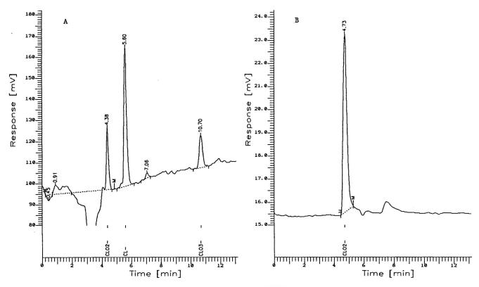
Figure 1. Chromatograms of representative 0.281 ppm chlorite, chloride, and chlorate standard solutions. (A) Conductivity detector. (B) Amperometric detector. Response scales are dissimilar.
