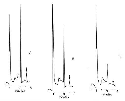
Figure 1. Liquid chromatograms of (A) wheat-flour extract, 3.5 mg bromide/kg; (B) lettuce extract, 1.7 mg bromide/kg; (C) and lettuce extract, bromide not detected. Arrow indicates retention time for bromide. The peak at 3 min is chloride.
