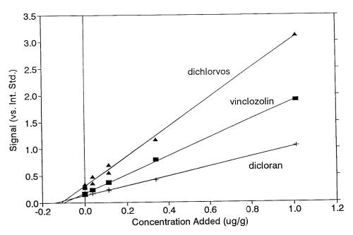
Figure 4. Determination of dichlorvos, vinclozolin, and dicloran in peach check sample using the method of standard additions.
