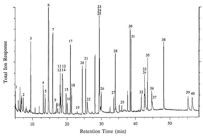
Figure 2. Typical GC/ITMS total-ion chromatogram of 40 pesticides fortified at 0.2 or 0.4  $\mu$ g/g in potato and extracted by SFE (Experiment 4A). The numbered peaks refer to the pesticides listed in Table 2.
