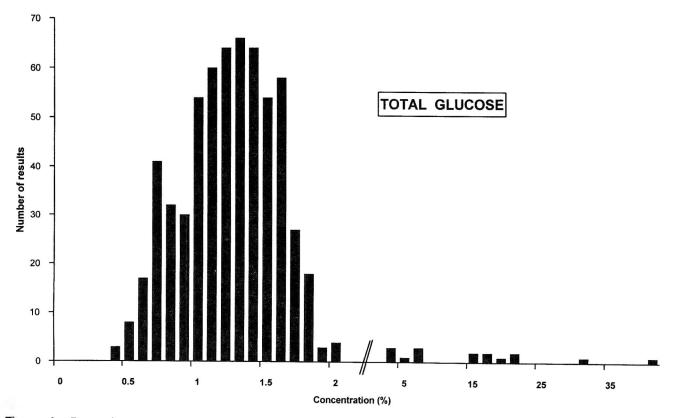
Figure 4. Determination of total glucose in commercial soluble coffee (619 results). Results for products with total xylose levels >0.40% were omitted.
