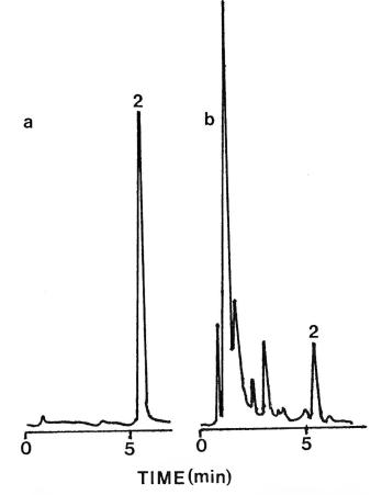
Figure 1. Liquid chromatogram of a TBZ standard (a) (peak 2 represents 0.84 ng TBZ injected) and an apple quencher sample (b) (peak 2 represents 0.21 ng TBZ injected).
