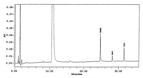
Figure 7. Chromatographic separation of amino acid derivatives in Vitalyte.
