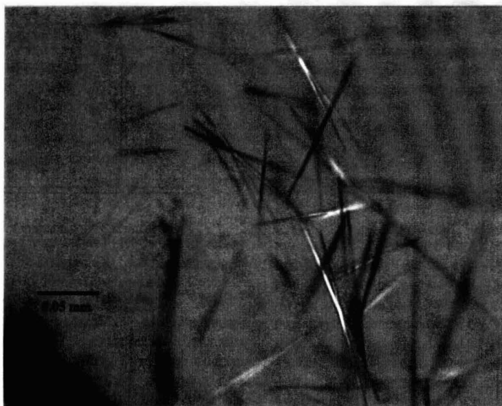
Figure 1b. The needle blade crystal form of dixanthylurea at 100 \times magnification.
