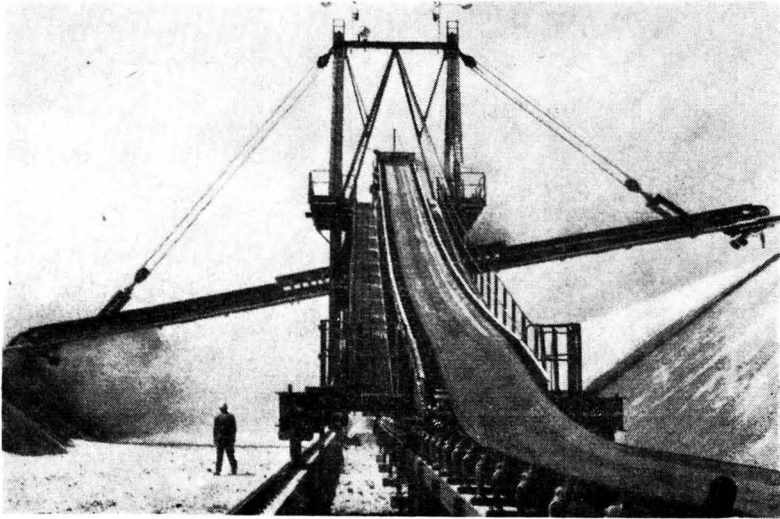
Fig. 3.—Method of Storing Raw Material: The Boom Travels Upwards as the Height of the Piles Increases.
