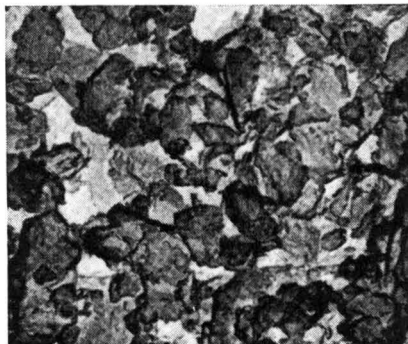
Fig. 4.—Electron-micrograph of a Grain of Ground \text{Ca}(\text{OH})_2 .
