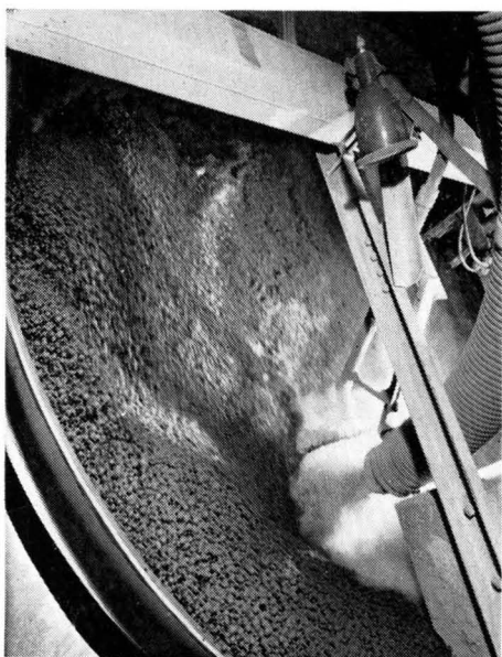
Fig. 12.—Nodules being formed in Noduliser Pan.
