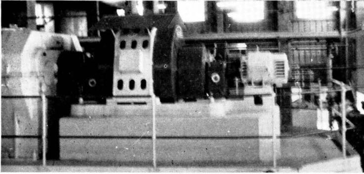
Fig. 20.—Mill Motor and Gear-box.
