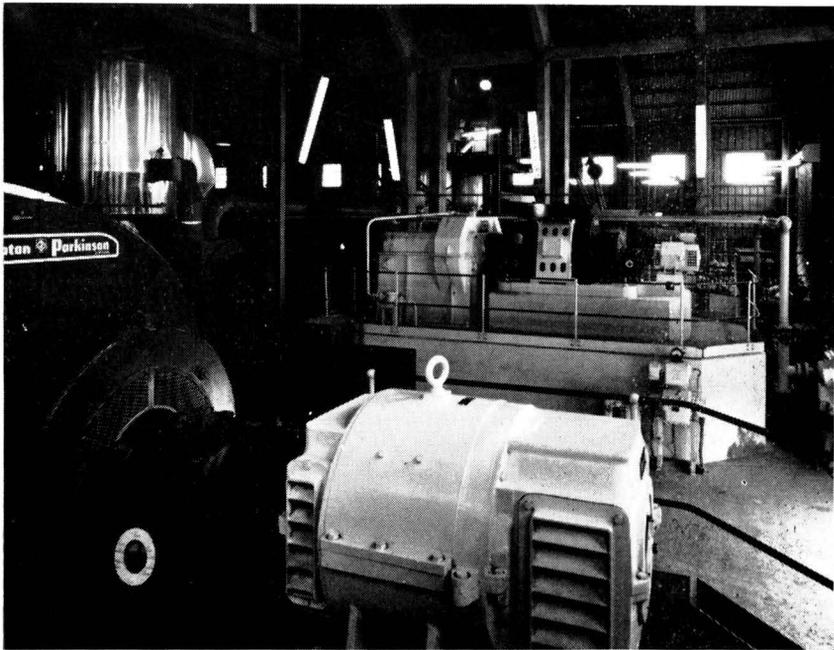
Fig. 19.—Mill Motor and Gear-box.
