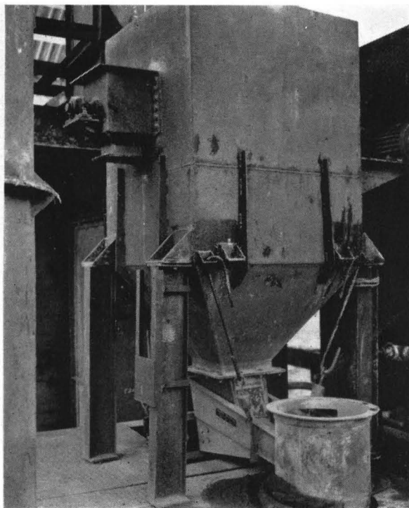
Fig. 5. Vibratory feeder controlling raw-meal feed to noduliser
