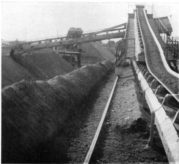
Fig. 6. (Right) Boom Trans- porter for stack- ing Raw Meal.
