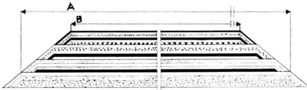
Fig. 5. Longitudinal section of pile. A = maximum travel of stacker. B = minimum travel of stacker.
